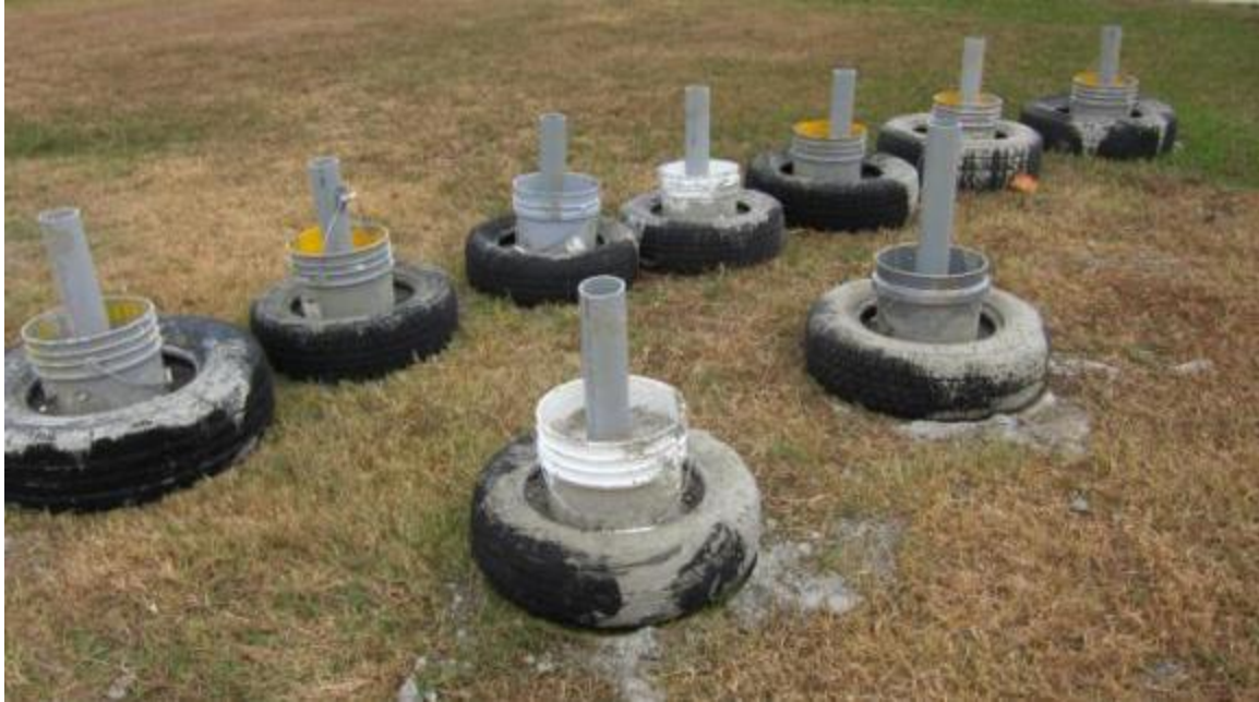
Figure 57. Concrete Tire Signpost Bases.
