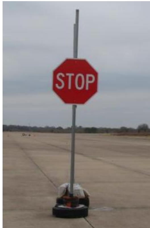
Figure 59. Sign with Clustered LEDs Visible for Lap A; Hidden behind a Standard 36-in. Sign (on Separate Post) for Lap B.
