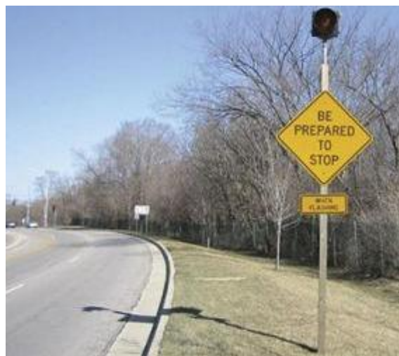
Figure 5. Example of Advance Warning with Beacon for a Signalized Intersection.
