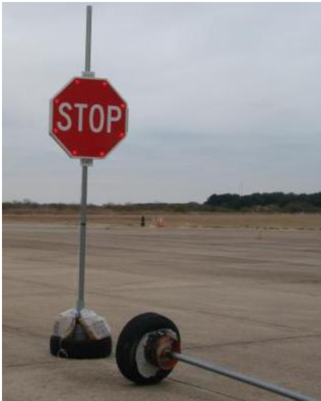
Figure 59. Sign with Clustered LEDs Visible for Lap A; Hidden behind a Standard 36-in. Sign (on Separate Post) for Lap B.
