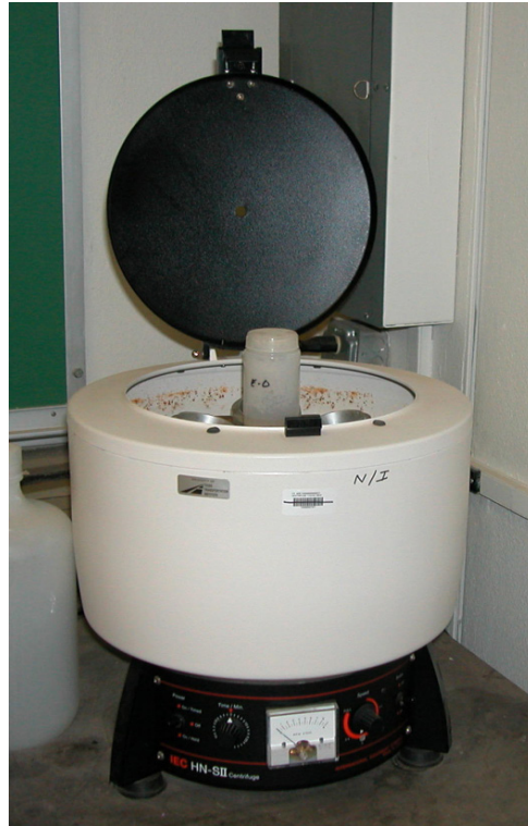
Figure B–3. Centrifuge Used to Aggregate the Sample prior to Decanting Supernatant.
