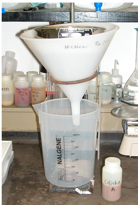
Figure B–4. Ringstand, Funnel, and Sieve Assembly Used for Sand Fractionation.
