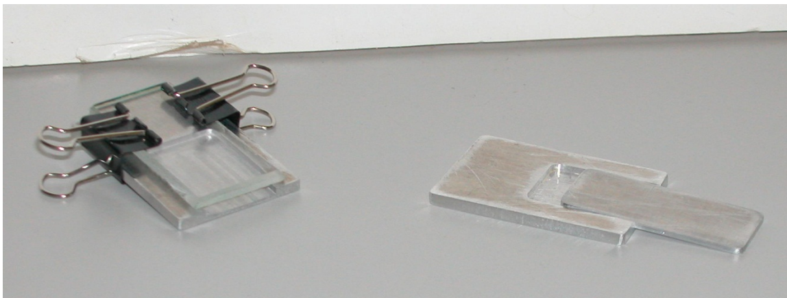
Figure B–13. Aluminum Holders Used for Side Loading Sand and Silt into X–Ray Unit.
