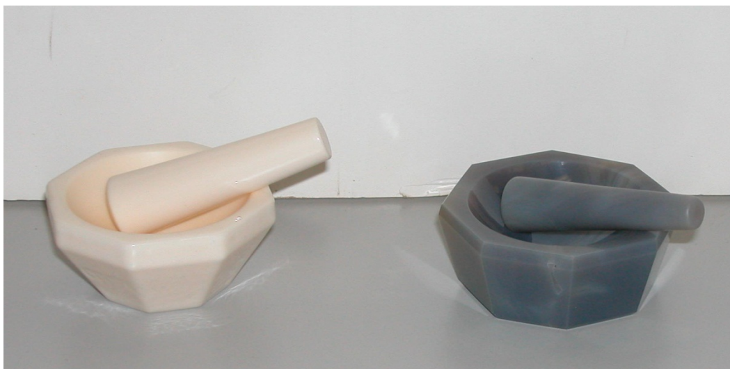
Figure B–12. Aluminum Oxide (left) and Agate Mortars and Pestles for Sand Reduction.
