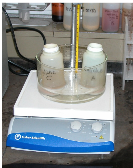
Figure B–1. The Bottles with Sample and 1N Na Acetate Solution Are Placed in Water Bath for Carbonate Removal.
