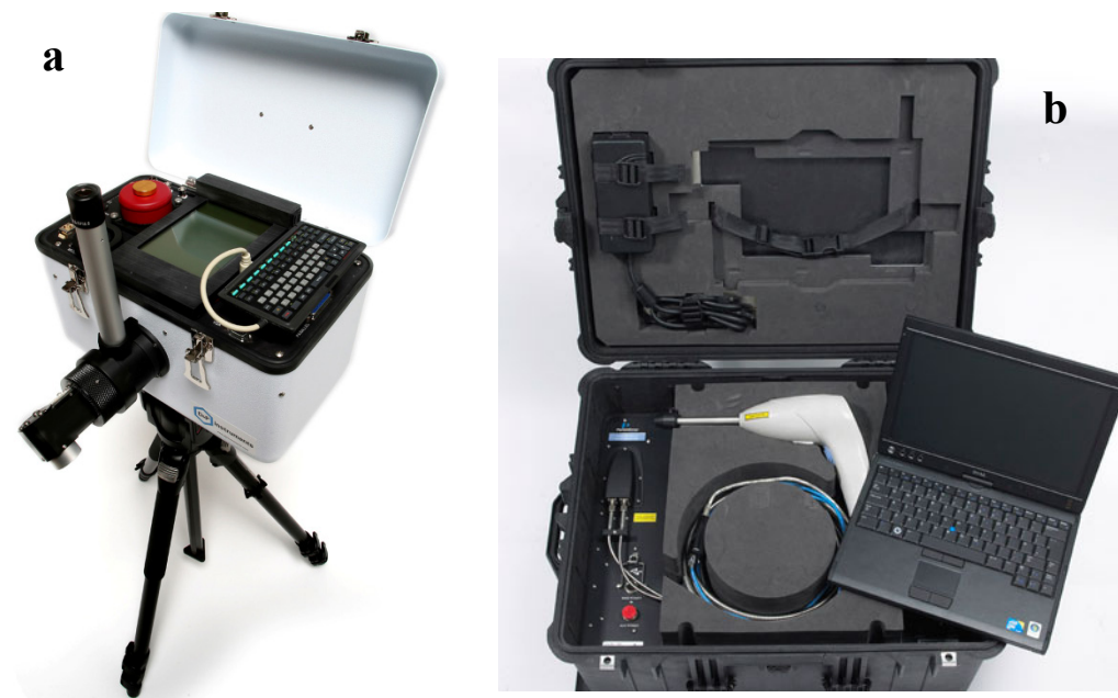
Figure 2.6. (a) A Hand–Portable FT–IR Spectrometer from D&P Instruments (Model 102) and (b) a Portable Raman Spectrometer (Raman IdenticCheck) from PerkinElmer.
