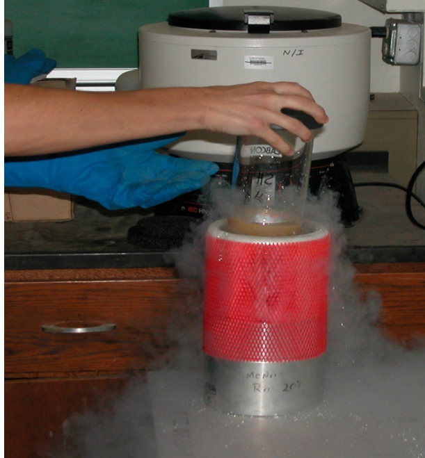
Figure B–10. Freezing Clay–Water Suspension Using Liquid Nitrogen.
