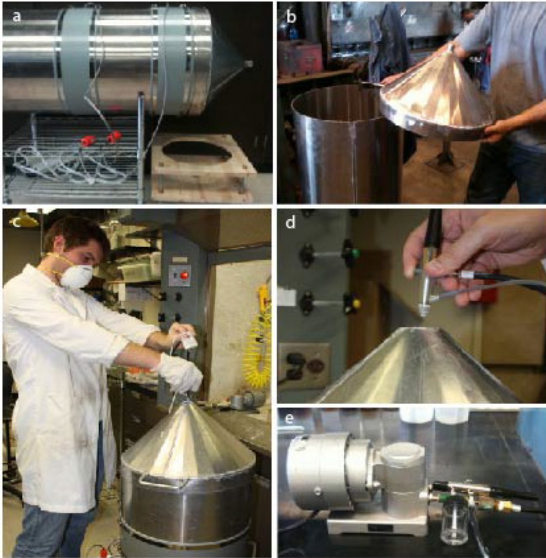
Figure E–1. Spray–Drying Procedure for Reducing Orientation Effects during Powder Diffraction.
