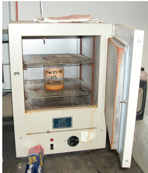
Figure B–6. Oven Set at 60°C for Drying Sand, Silt, and Coarse Clay Fractions.
