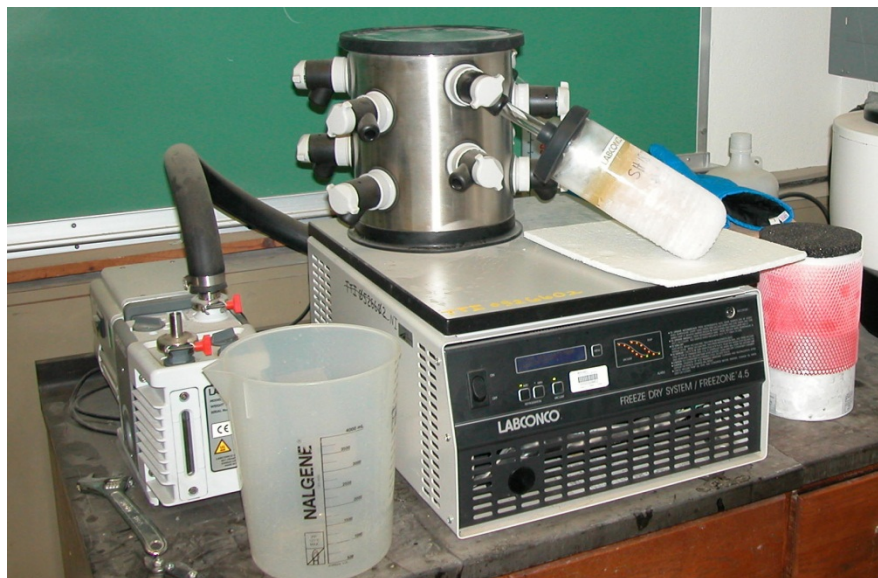
Figure B–11. White Coating of Ice on the Flask, Indicative of a Successful Freezing Job.
