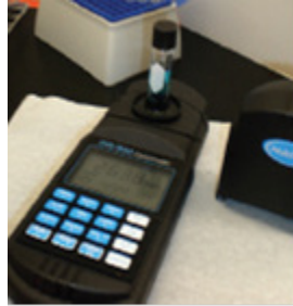
Figure 4.11. A Sample Tube Is Inserted into the Tube Adapter.
