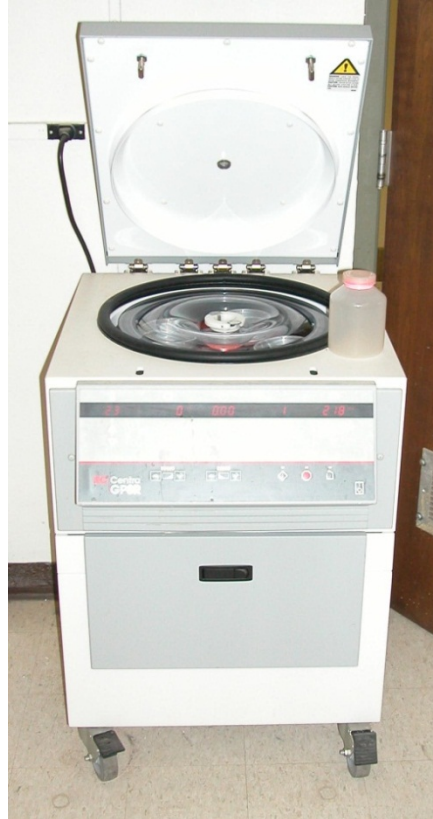
Figure B–5. IEC Centra GP8R Centrifuge Used to Separate Silt and Clay Fractions.
