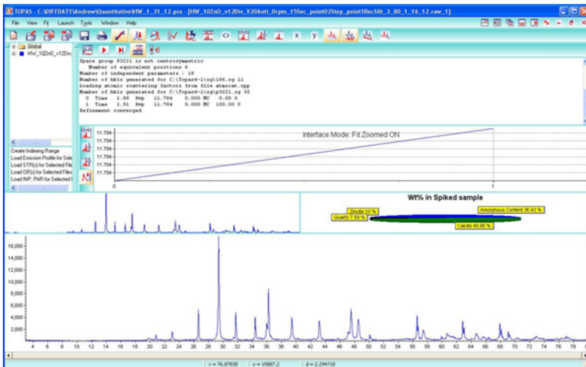
Figure 4.5. Bruker's TOPAS Program Interface for Rietveld Analysis from Crystal Structures.
