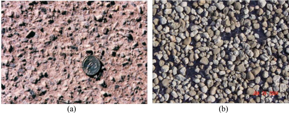
Figure 2.2. (a) Effect of Fines in Seal Coat Aggregate Surface with Excess Fines after Sweeping (b) Surface of Seal Coat with Clean Aggregate.
