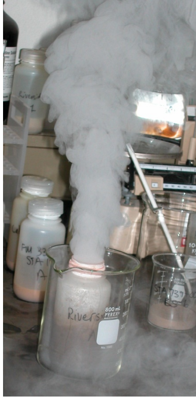
Figure B–2. Removal of Organic Matter Often Results in a Violent Reaction.
