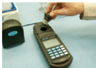
Figure 4.10. Installation of the Tube Adaptor.
