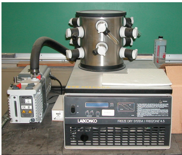
Figure B–9. Freeze Dryer Used to Remove Water from the Fine Clay Fraction of Samples.
