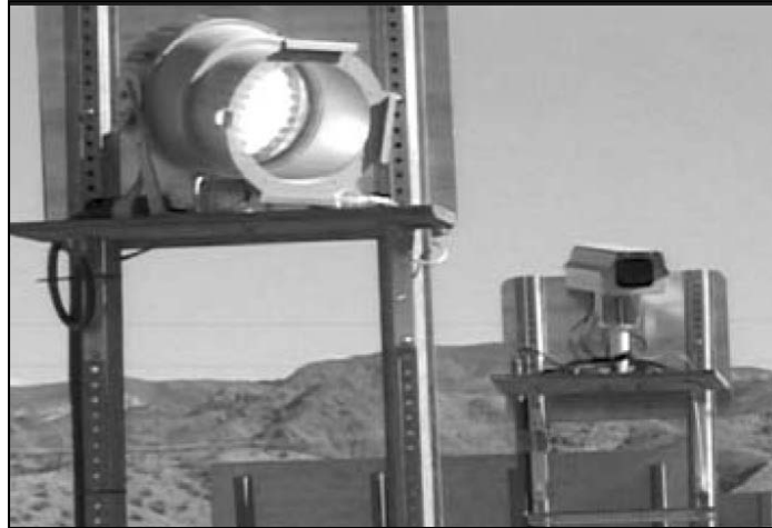
Figure 29. Light and Camera Used for License Plate Recognition (57).
