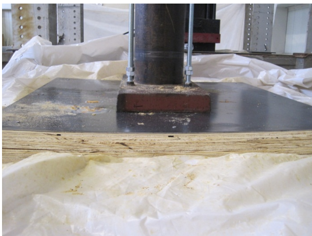
Step 11. Conduct static load test.
