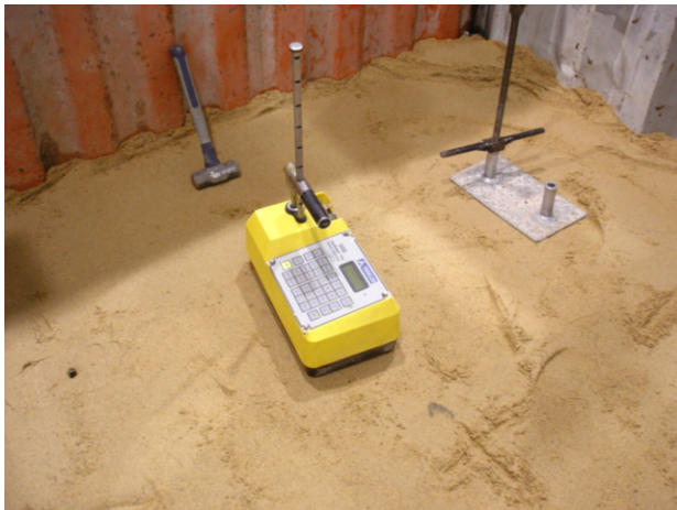
Step 3. Measure density and moisture content.
