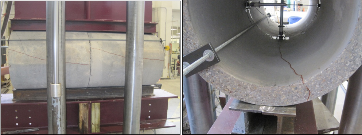
Figure 61. Propagation of Crack of the Jointed Concrete Pipe.
