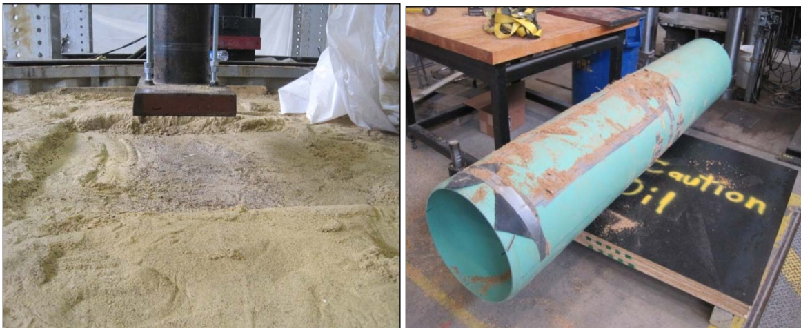
Figure 47. Visual Inspection after Fatigue Test of Unjointed PVC Pipe.
