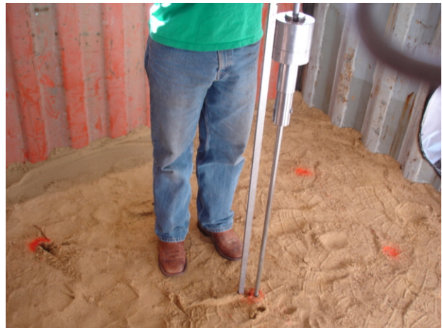
Step 4. Measure soil modulus using DCP.
