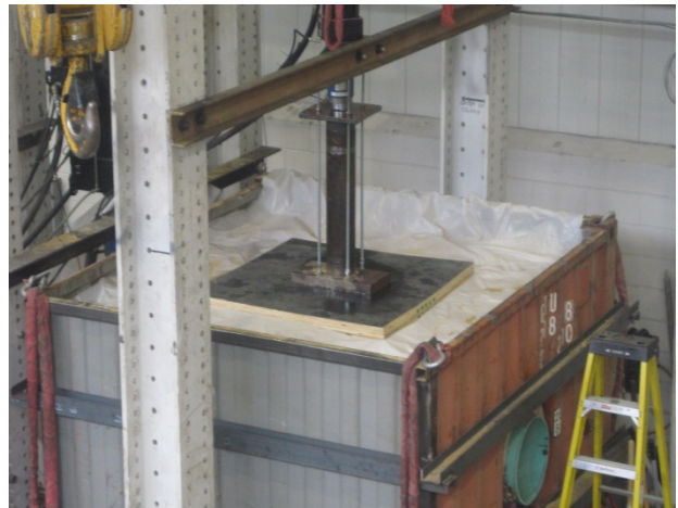
Step 10. Set up loading frame and plate.
