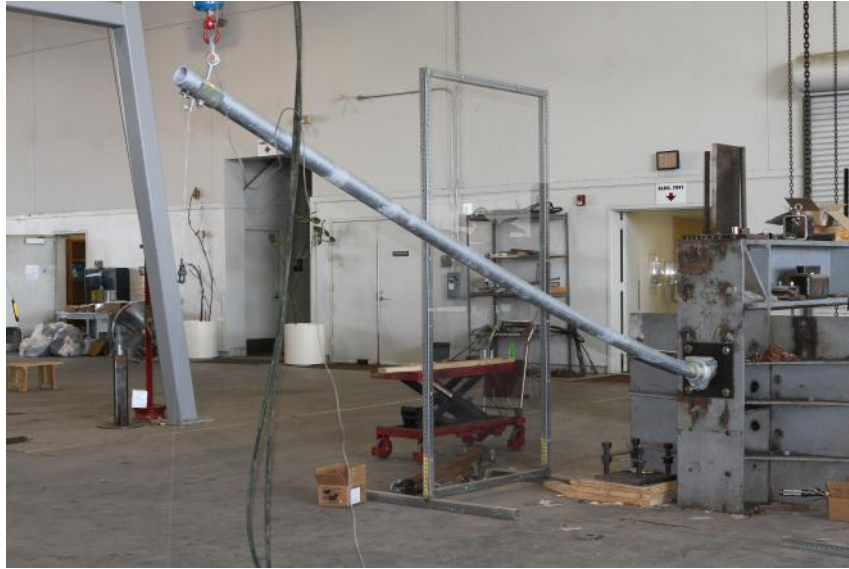
Figure 11.15. Schedule 80 Pipe Support Static Test Setup at Maximum Load.
