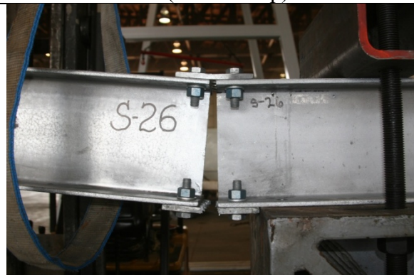
(e) Fuse Plate Connection after Failure ( \frac{3}{8} -inch Gap)
