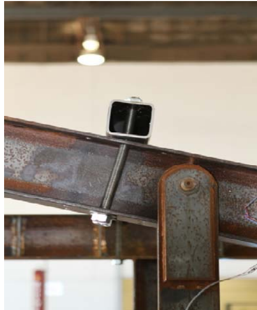
Figure 7.8. Static Test of HSS3×3×1/8 with Through Bolt Connection.
