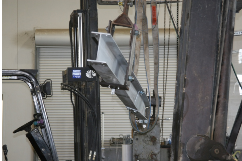
Figure 5.13. W8×18 Support at Maximum Load (S3).
