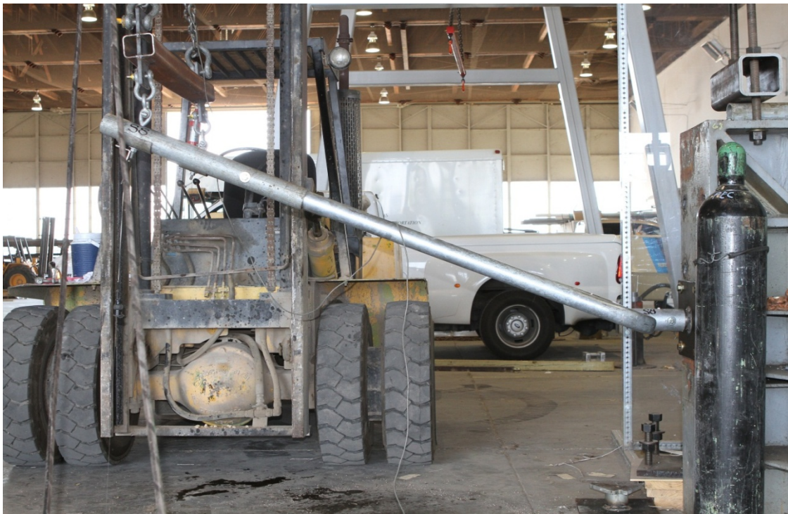
Figure 11.20. U-Bracket Static Test Setup at Maximum Load.
