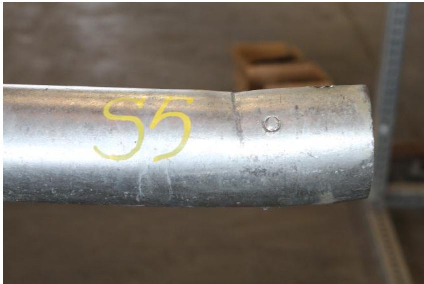
Figure 11.16. Deformation to Schedule 80 Pipe Support.
