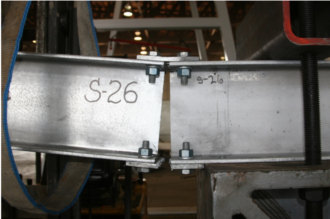
Figure C9. Test Sample S26 after Fuse Plate Rupture.
