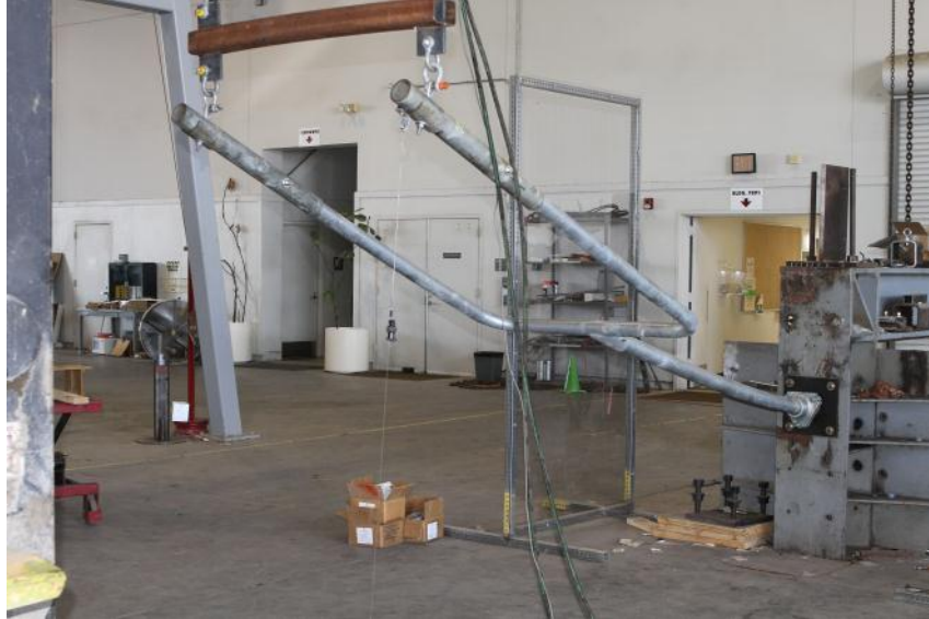
Figure 11.12(a). Image of U-Bracket Installation Static Test Setup at Maximum Load.
