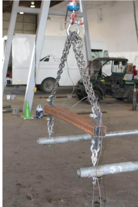
Figure 11.11. Image of U-Bracket Load Application.
