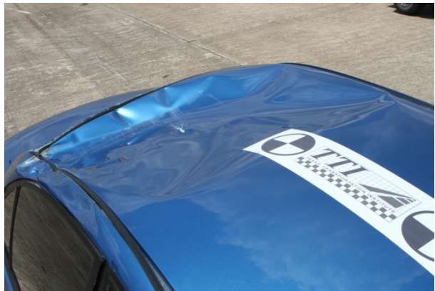
Figure 9.42. Vehicle Roof Deformation after Test No. 463631-2.
