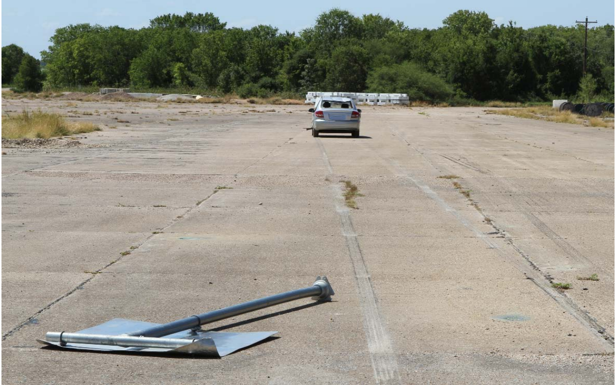
Figure 9.55. Position of Sign Support/Vehicle after Impact for Test No. 463631-3.
