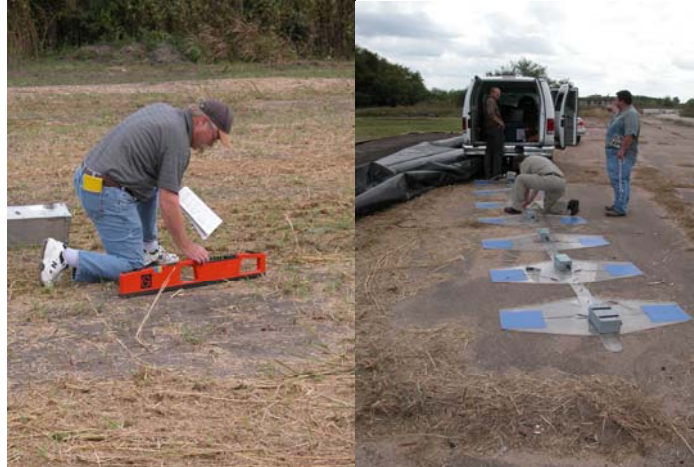
Figure 1.5. Two Devices [EM-38 (Left), PACES (Right)] Tested at Riverside Campus for Sulfate Detection.
