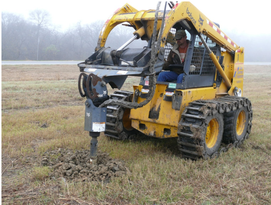
Figure 5a.15. Bobcat with 9-Inch Auger Used to Collect Soil Samples to a Depth of 4 Ft.
