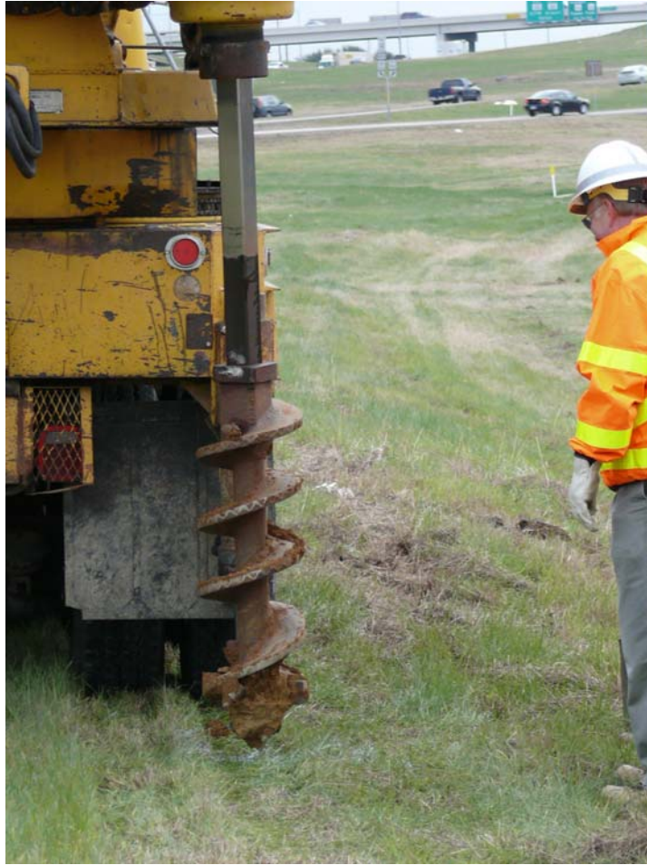
Figure 5a.8. Auger Used to Collect Soil Samples Every 1 Ft to a Depth of 4 Ft in Areas of Contrasting Conductivity.
