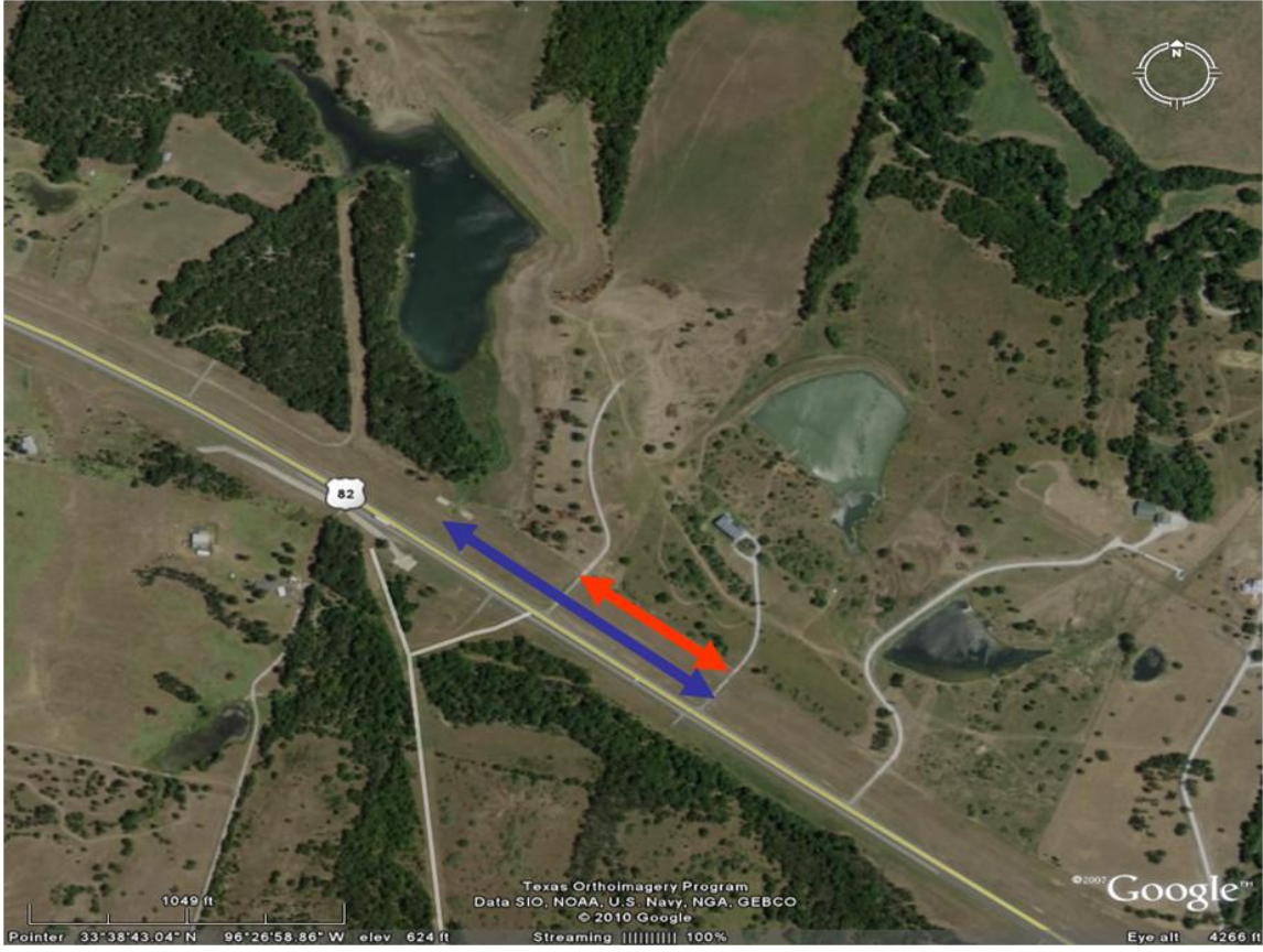
Figure 5a.26. Aerial View of US 82 Project Shows High Sulfate Zone (Red Arrow) and Extent of Data Collection (Blue Arrow).
