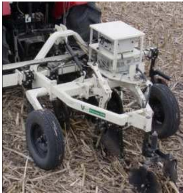
Figure 1.12. Veris VIS-NIR Spectrophotometer Used to Measure Soil Carbon.
