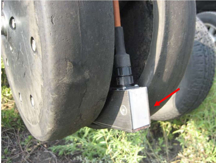
Figure 5b.2. NIR Detector (Red Arrow) Attached between the Rubber Wheels.
