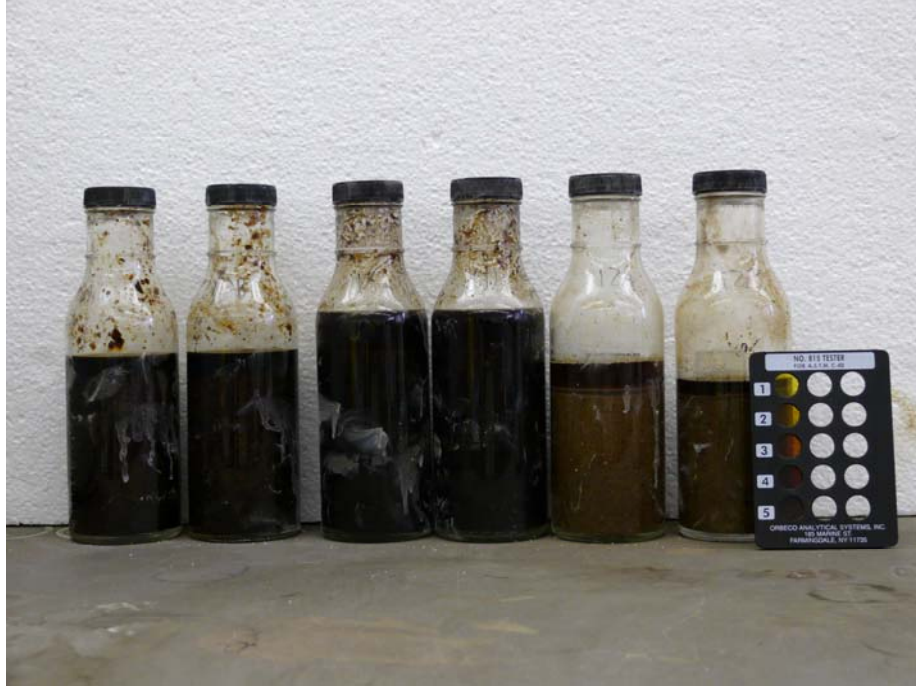
Figure 1.11. Colorimetric Technique (Tex-408-A) Can Yield Artificially High Organic Contents.
