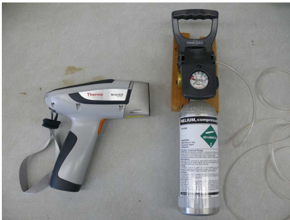
Figure 2.1. Niton XL3t Handheld XRF Detector with He Purge System.
