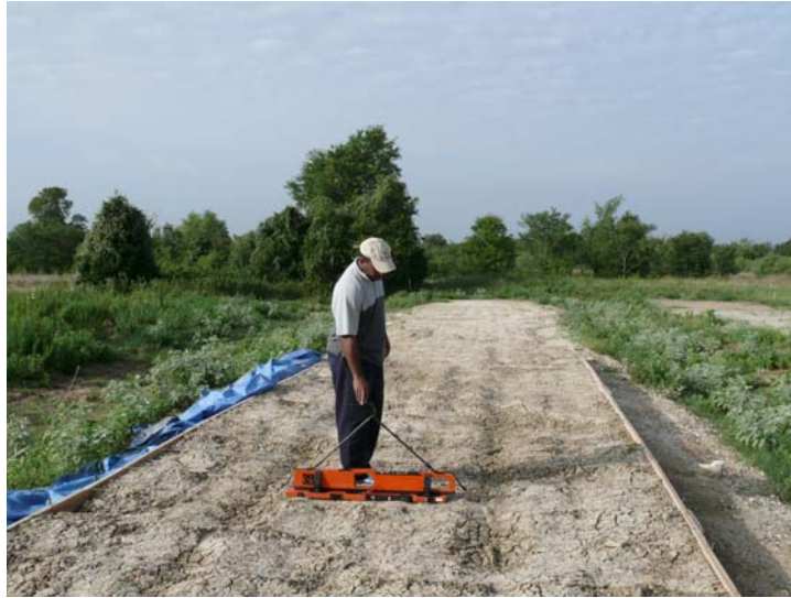
Figure 3.3. EM-38DDRT Used to Measure Electromagnetic Properties of Soil.
