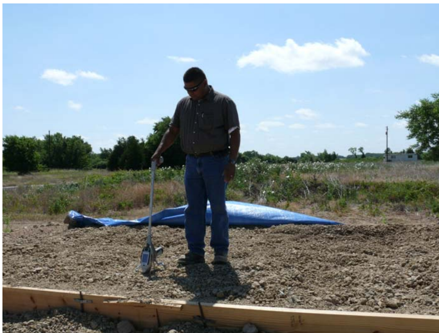
Figure 1.10. Portable XRF Used to Detect Sulfur in Experimental Site at Riverside Campus, Texas A&M.
