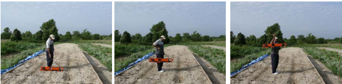
Figure 3.6. EM-38DDRT Data Collection at Heights of 0, 2, and 4 Ft above Ground.
