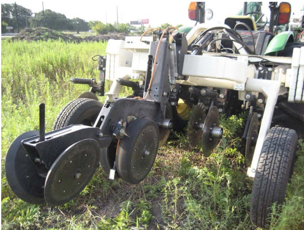
Figure 5b.1. Black Implement NIR Device that Is Attached to Veris 3150.
