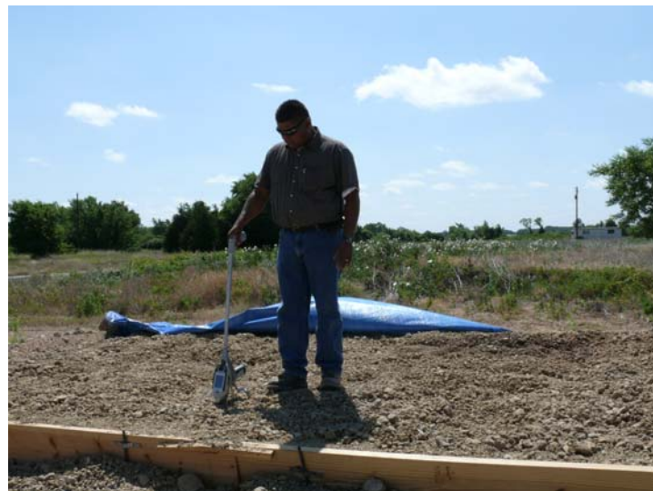
Figure 3.4. Portable XRF with Extendapole Used for Measurement in the Field.
