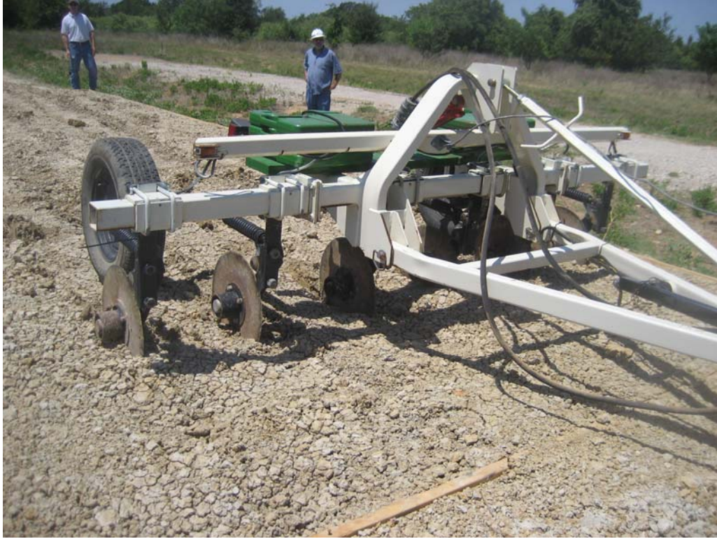
Figure 3.5. Veris 3150 Conductivity Device Used to Measure Conductivity of the Soil.
