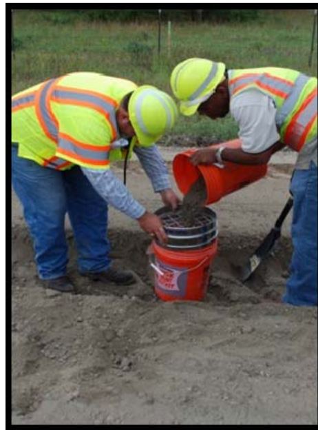
Figure 2.2. Checking Field Pulverization by Sieving.
