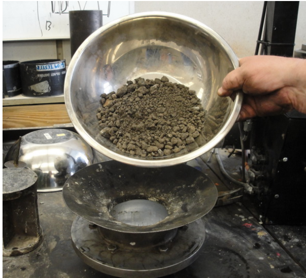
Figure 4. Placement of the Material into the Mold Using the Wide-Mouthed Funnel.
