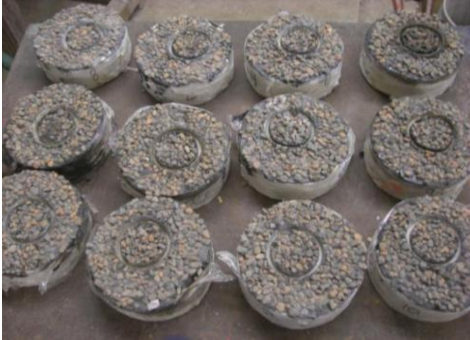
Figure 3.12. Laboratory Specimens Cut Using 2-In. Core Barrel prior to Bond Strength Testing.
