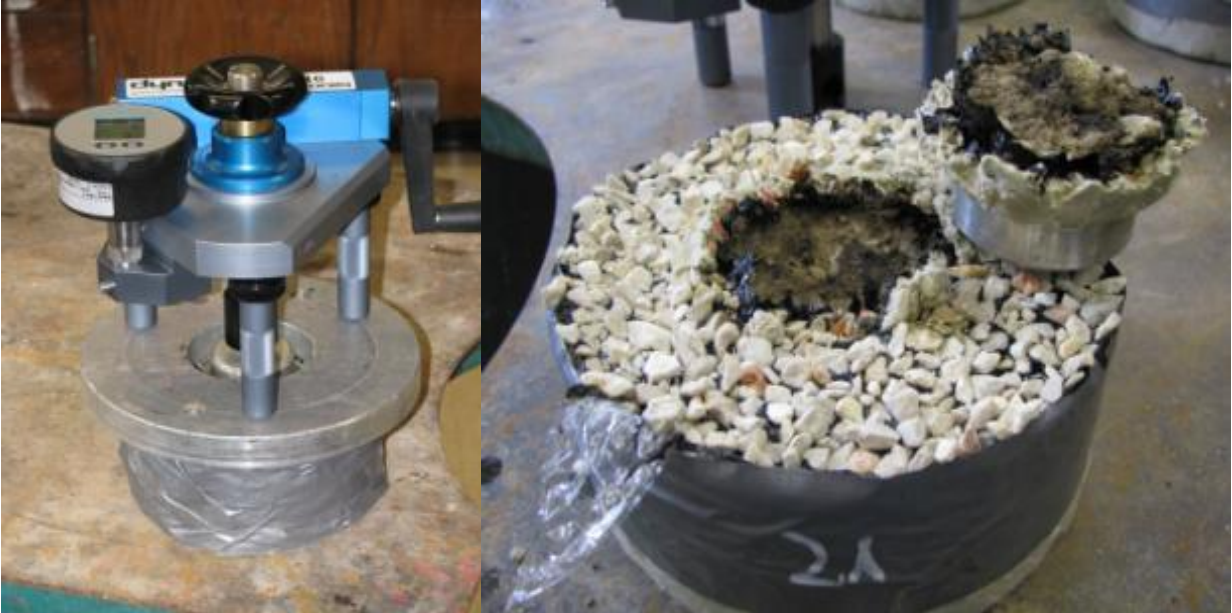
Figure 3.1. Surface Treatment Bond Test Equipment and Tested Lab Specimen.
