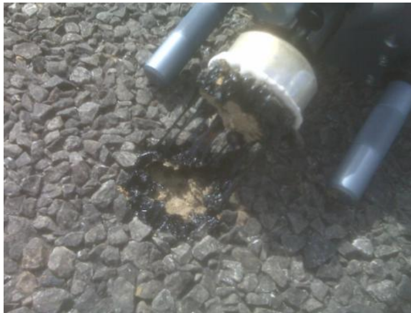
Figure 3.19. Surface Treatment Bond Testing on FM 2502.
