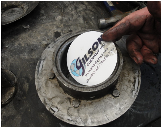
Figure 3. Set-Up for Texas Gyratory Compactor Mold.
