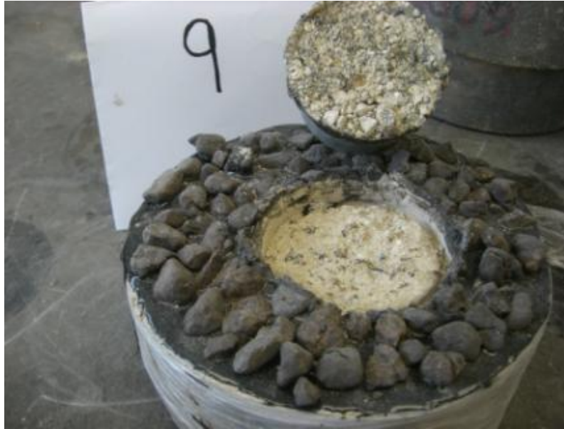
Figure 3.9. Failure Plane of Surface Treatment Bond Test when No Prime Was Used (Failure at Surface Treatment/Base Interface).
