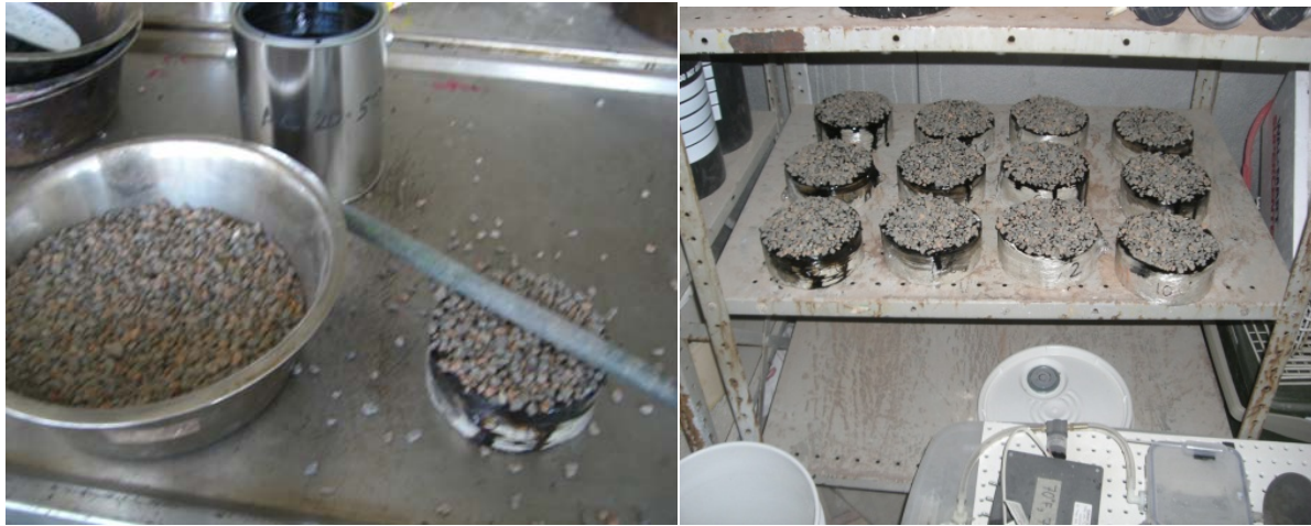
Figure 2.5. Application of Surface Treatment to Primed Base Samples.
