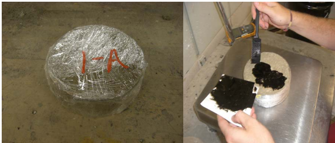
Figure 2.4. Application of Prime to Base Sample.
