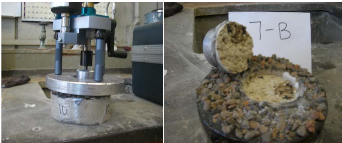
Figure 2.8. Sample in Testing Apparatus and after Failure.
