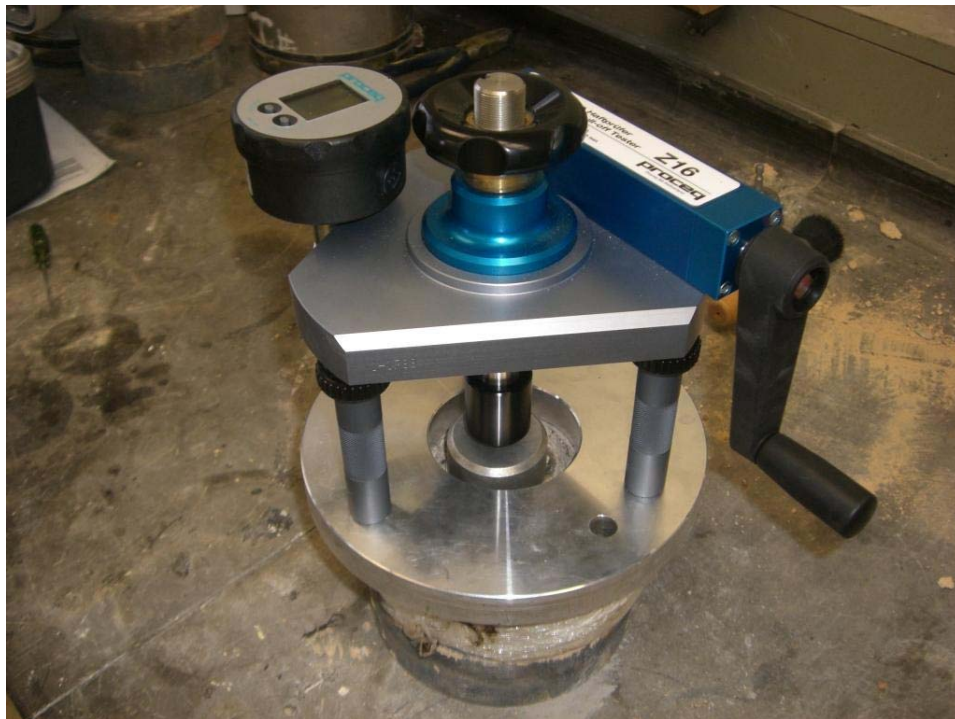
Figure 2.3. Photo of Direct Tensile Bond Test Apparatus.
