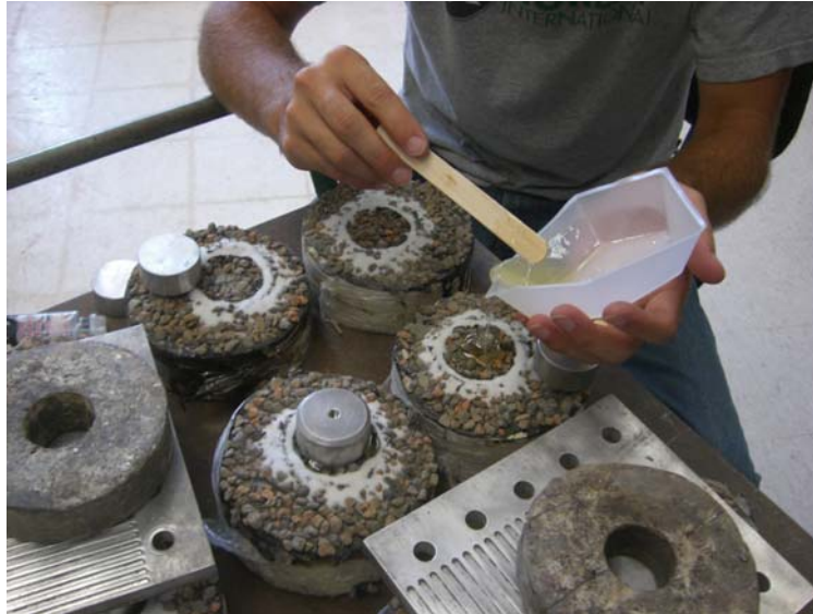
Figure 2.7. Gluing Metal Disks to Surface Treated Base Samples.
