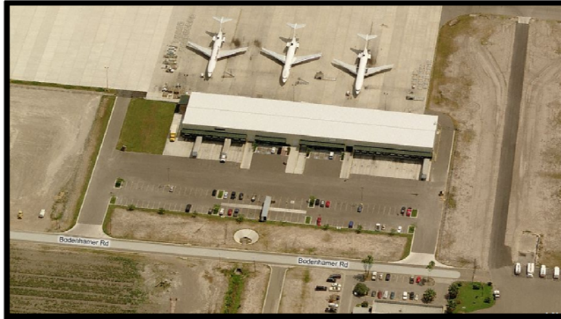
Figure 165. Freight Facility with Space for Truck Backing Maneuvers.
