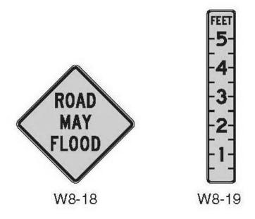
Figure 3. Road Flooding Conditions Warning Signs in National MUTCD.
