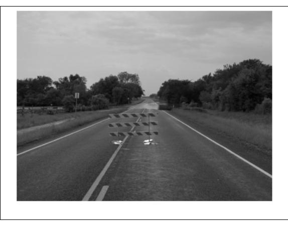
Figure 18. Example of Use of Temporary Barricade to Alert Drivers to Flooded Roadway Conditions.
