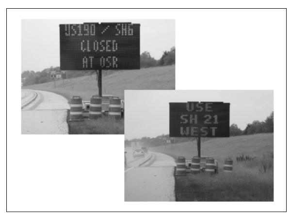
Figure 20. Example of Use of Portable Dynamic Message Sign to Alert Drivers to Flooded Roadway Conditions.
