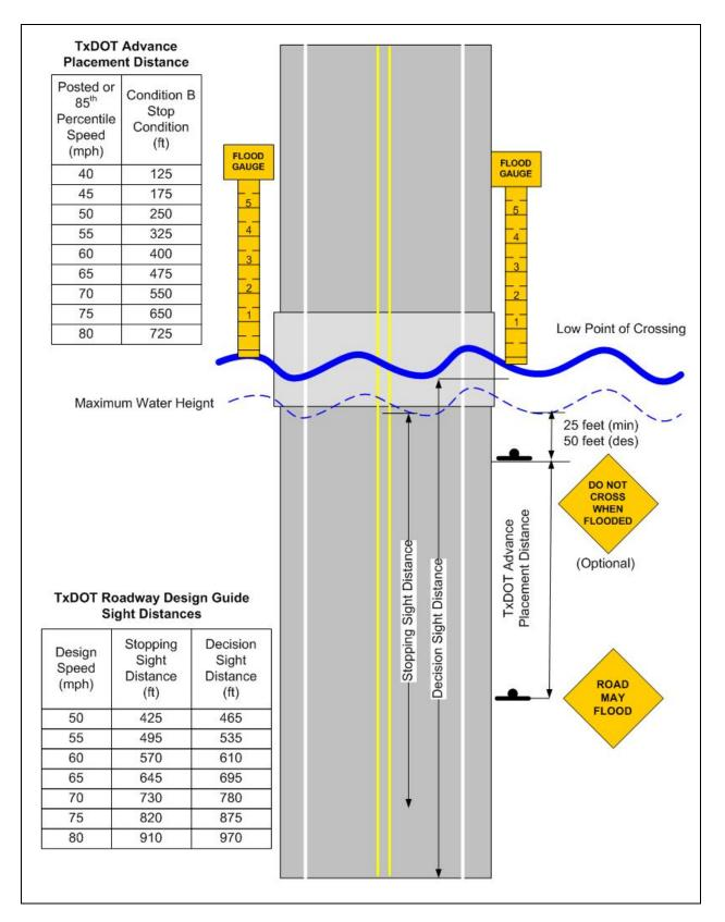
Figure 42. Candidate Signing Layout for Flood-Prone Crossing—Static Signs Only.
