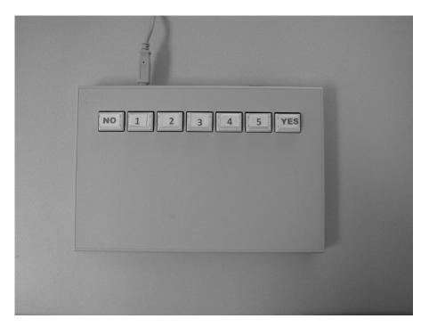
Figure 24. Button Box Used for Participant Response Entry.
