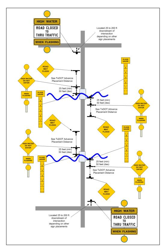
Figure 45. Candidate Signing Layout for Roadway with Multiple Flood-Prone Crossings.
