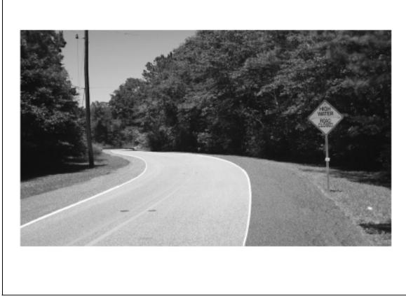
Figure 14. An Example of a Sign Treatment in Advance of Flood-Prone Crossing.
