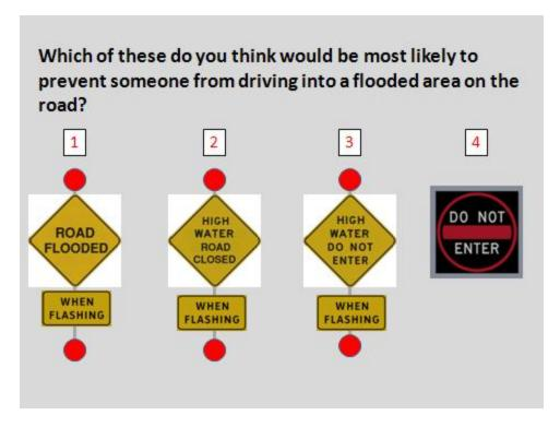
Figure 40. Active Warning Signs Tested in Driver Preference Study.
