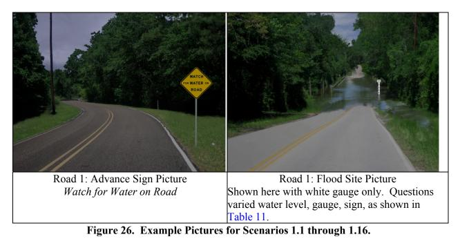
(the pictures shown feature the advance warning sign and the white flood gauge that are the current *TxDOT* standard treatment for flood-prone sites).
