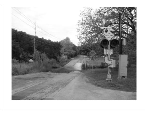
Figure 22. Example of Flood-Prone Crossing with Automated Gate.
