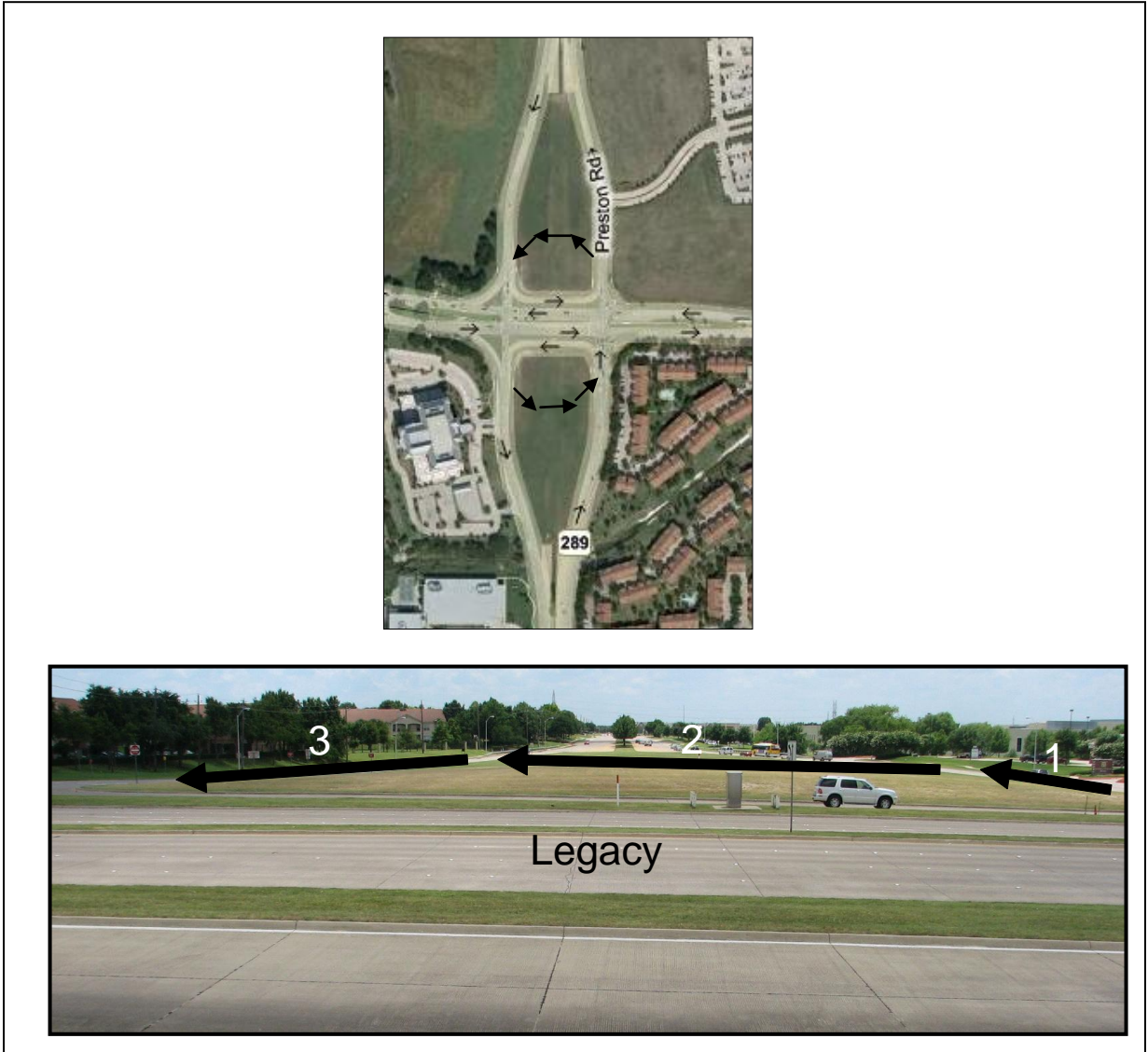
Figure 59. Proposed “Median Left-Turn” Concept.
