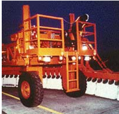
Figure 19. Example of Moveable Barrier and a Barrier Transfer Machine.
