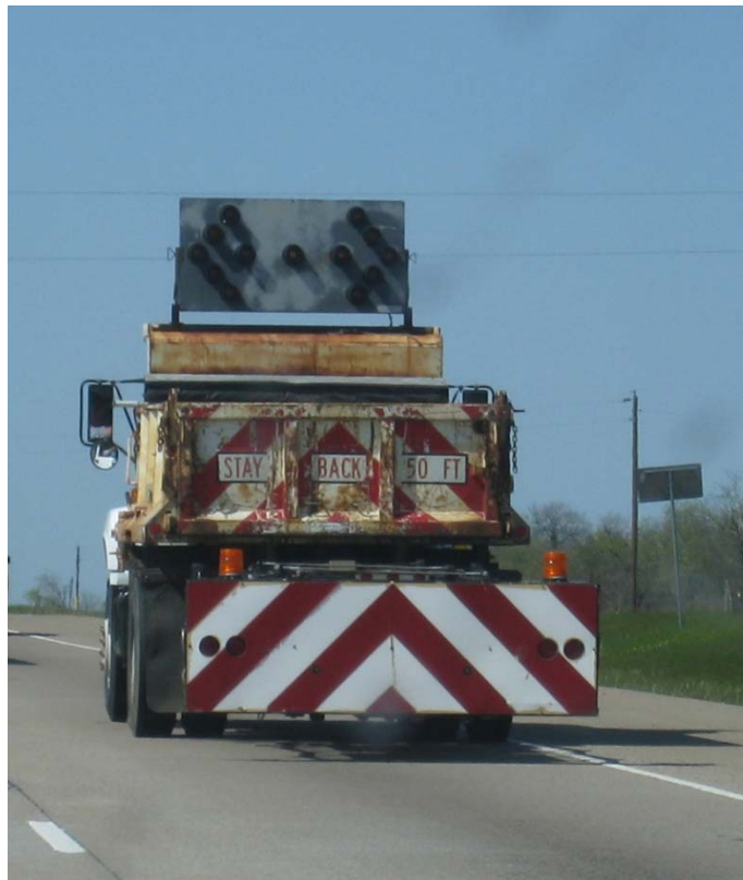
Figure 22. Example of a TMA in Use during a Mobile Operation.
