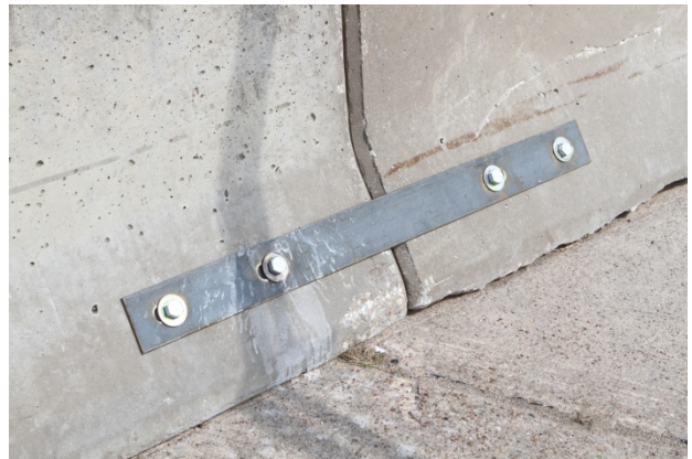
Figure 5. TxDOT PCTB with Sign Support Assembly and Steel Strap Connections before Test No. 461430-1.
