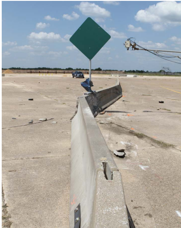
Figure 8. After Impact Vehicle Position for Test No. 461430-1.
