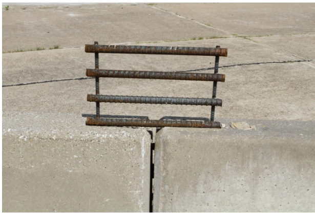
Figure 5. TxDOT PCTB with Sign Support Assembly and Steel Strap Connections before Test No. 461430-1.
