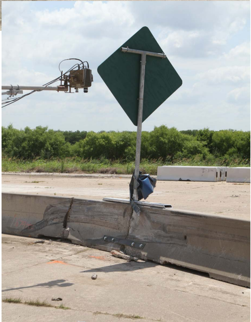
Figure 9. Installation after Test No. 461430-1.
