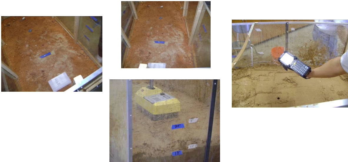
Figure 18. Data Collection Using Motorola Reader and Nuclear Density and Moisture Content Measurements Apparatus.
