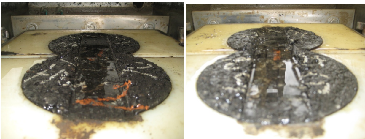
Figure 4-3. Type D 5.2% AC (3.1 mm) and 5.5% AC (4.1 mm) HWTT Specimens (ATL).
