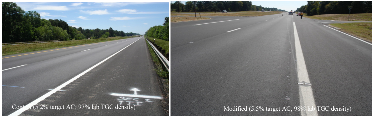
Figure G-1. View of the Test Sections – No Visible Surface Rutting or Cracking – ATL. (After 5 Months; Oct 2010).
