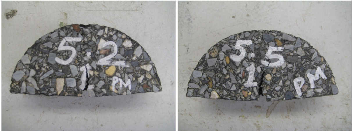
Figure 4-6. Type D 5.2% AC (124 psi) and 5.5% AC (100 psi) SCB Specimens (ATL).
