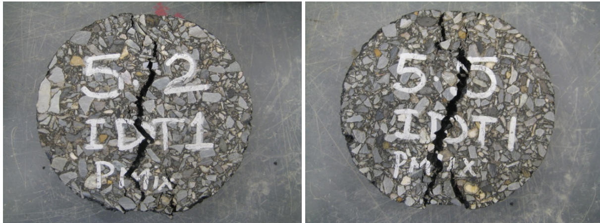
Figure 4-5. Type D 5.2% AC (126 psi) and 5.5% AC (104 psi) IDT Specimens (ATL).
