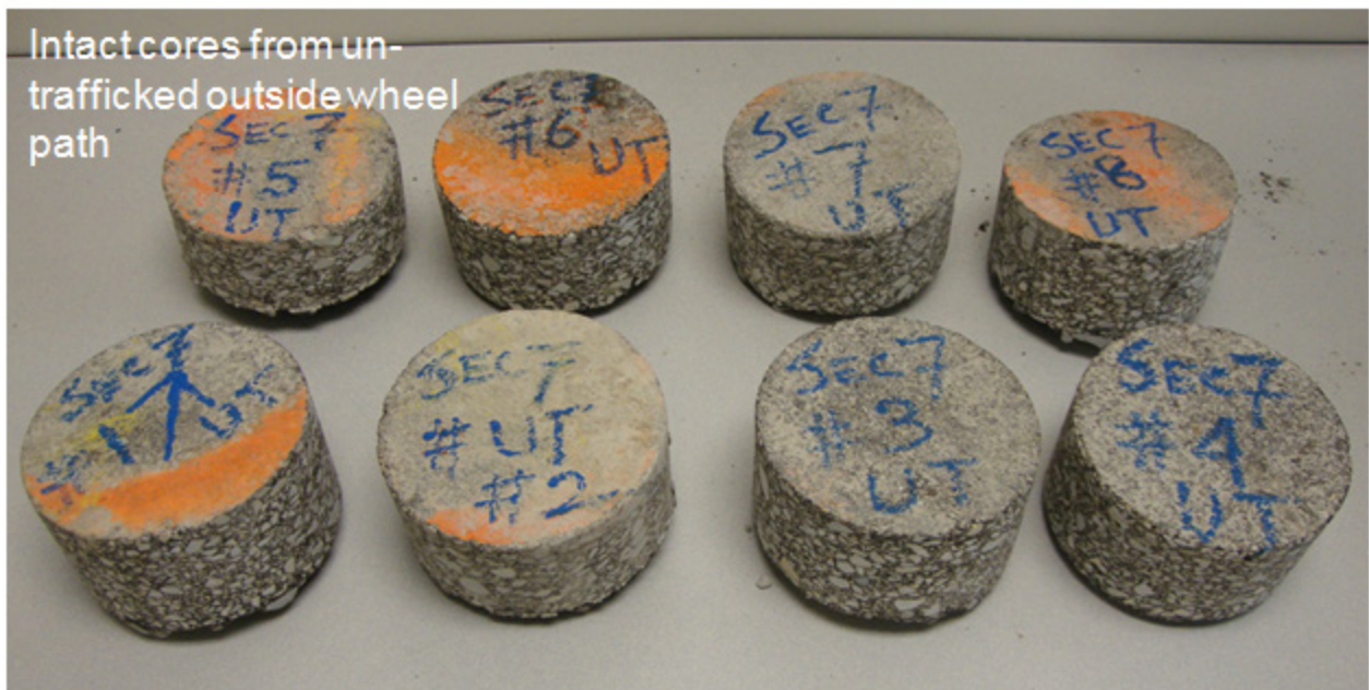
Figure 5-10. Cracked and Uncracked Cores from Modified Section 7.
