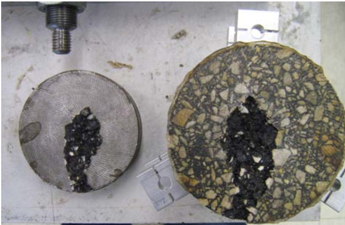
Figure 5-3. Example of End Cap Failure.
