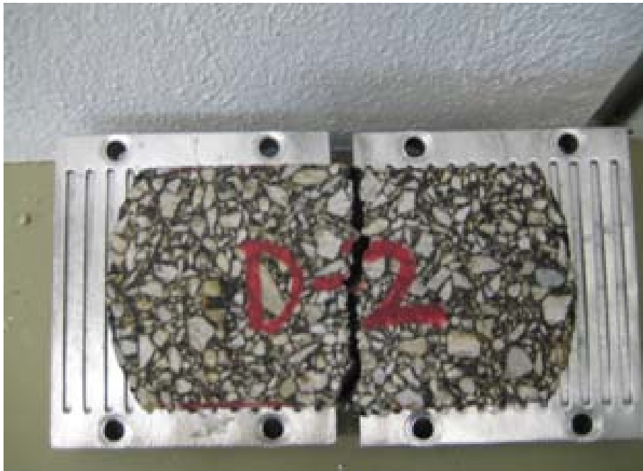
Figure 5-1. Example of Typical OT Crack Failure with a Single Crack.
