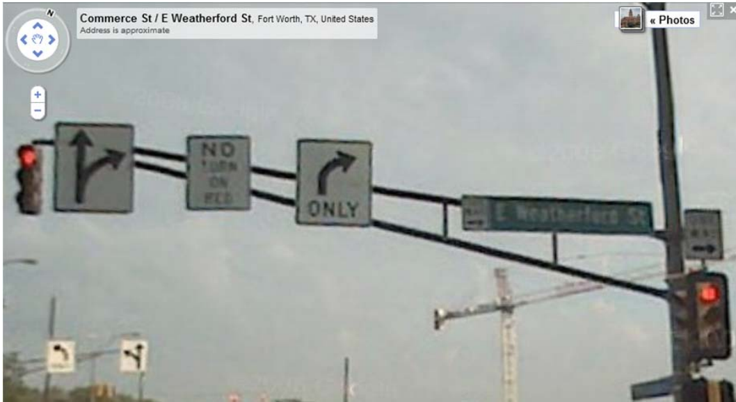
Figure 7-2. Advance Overhead Sign for Dual Right-Turn Lane.
