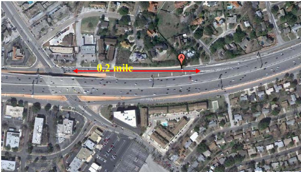
Figure 5-6. Illustration of Short Deceleration Distance as a Contributor to Rear-End Crashes (Babcock Road at WB IH-410, San Antonio).
