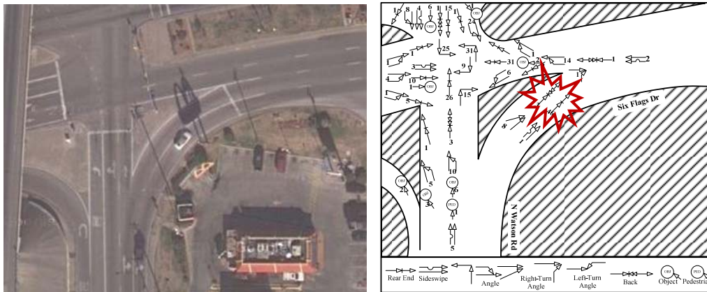
Figure 5-3. Rear-End Crash Hot Spots at Six Flags Drive at SH 360.
