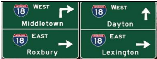
Figure 108. Example of Guide Signs Using a Right-Angled Arrow vs. a Straight Arrow.
