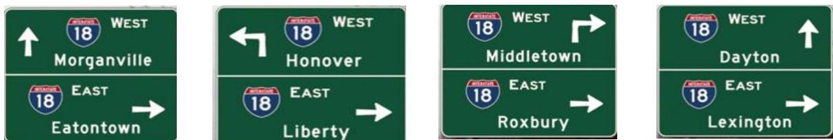
Figure 35. Examples of Arrow Concepts for Cross-Street Approach Signing to an Unsignalized Intersection or Interchange.
