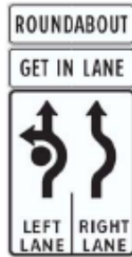
Figure 11. British Columbia Ministry of Transportation R-507 (ROUNDABOUT) & R-508 (GET IN LANE) Name Tabs. (11)
