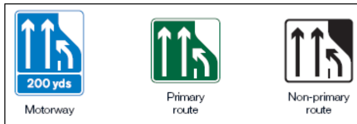
Figure 38. United Kingdom Trap Lane and Additional Lane Use Ahead Signs with a Lane Reduction Taper. (22)
