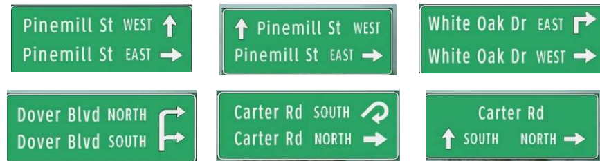
Figure 34. Examples of Arrow Concepts for Frontage Road Approach to an Unsignalized Intersection or Interchange.
