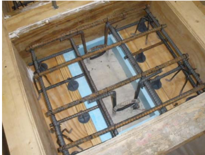
Figure 3.7 Photograph of reinforcing of a CIP shear test specimen..
