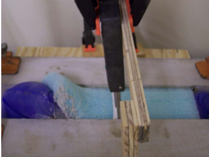
Figure 4.12 A lateral pressure test specimen at failure.
