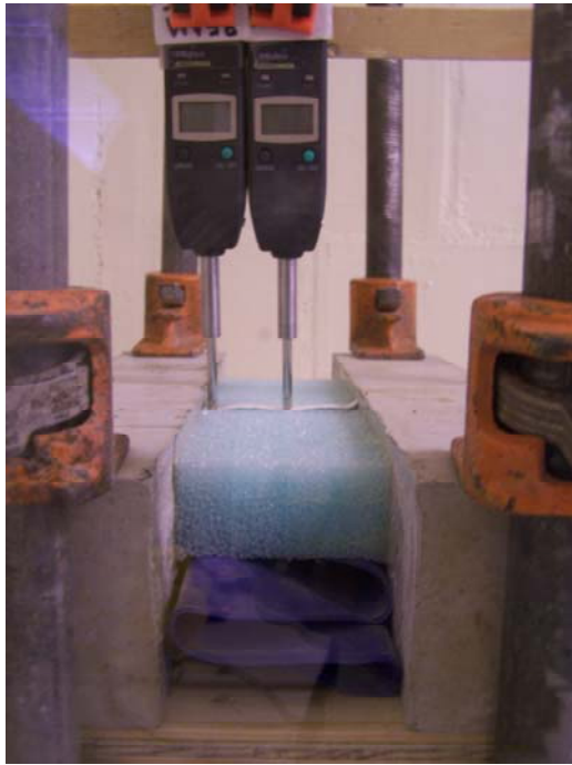
Figure 4.11 Experimental setup for the lateral pressure test.
