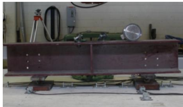
Trailing wheel load over two panels
