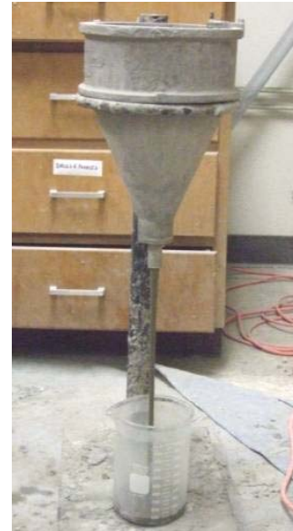
Figure 4.1 Efflux cone test.
