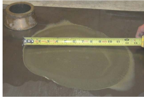
(b) Flow cone showing signs of segregation
