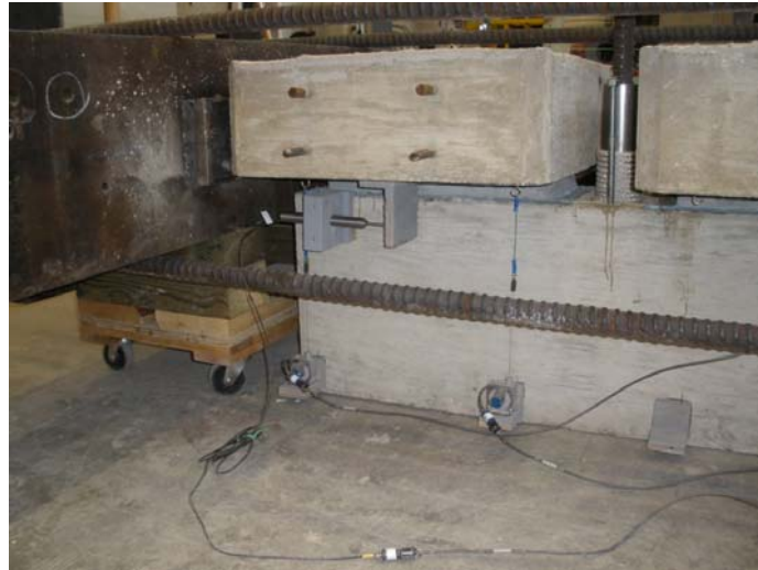
Figure 3.8 Photograph of LVDTs and string potentiometers connected to a shear test specimen.
