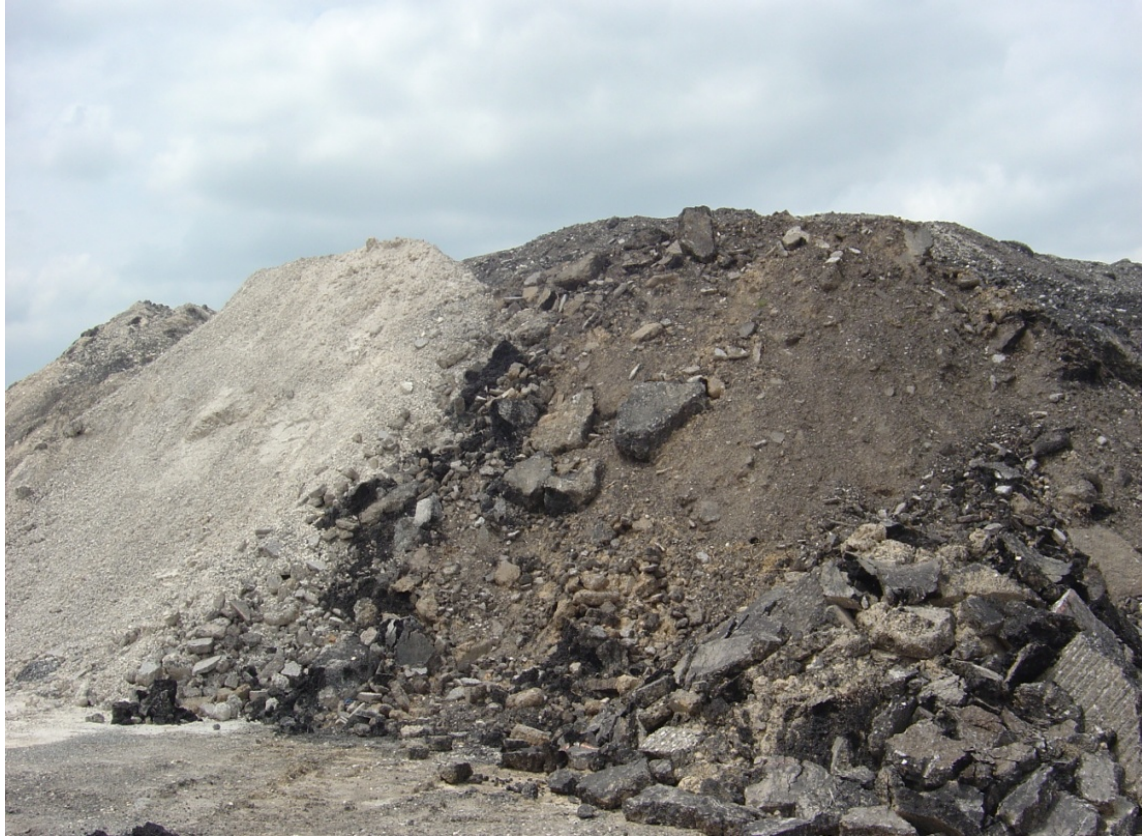
Figure 2-6. RAP Stockpile Contaminated with Subgrade Soil.
