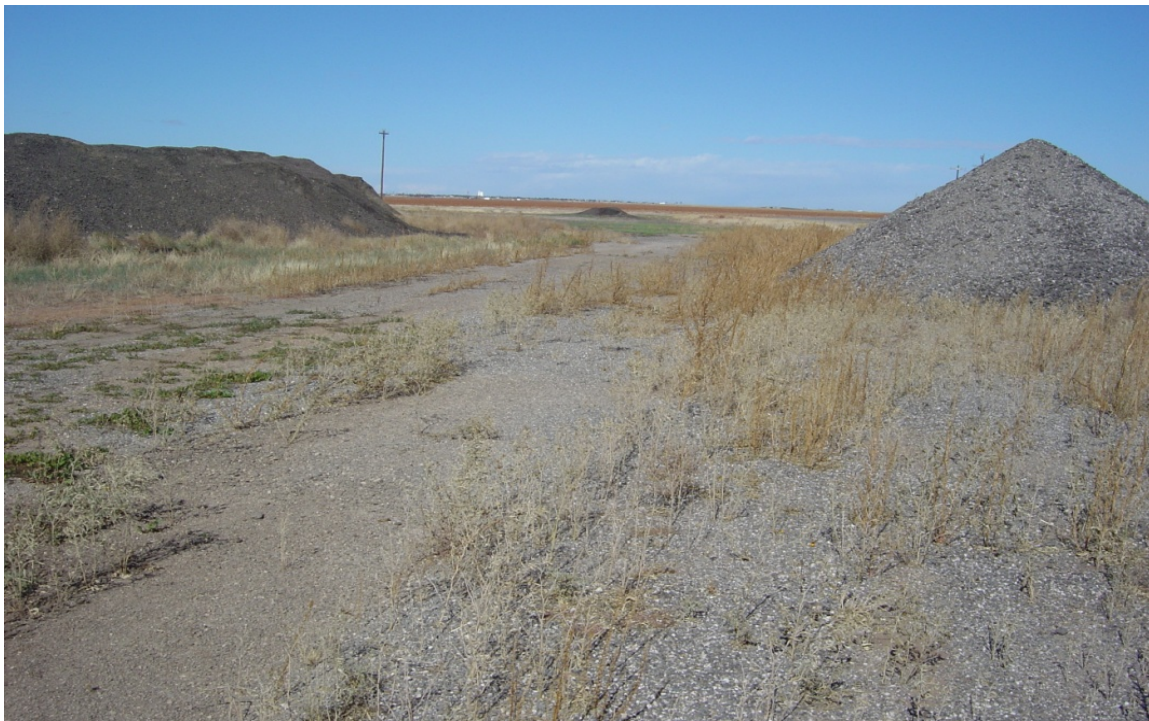
Figure 2-1. Two Separated RAP Stockpiles.
