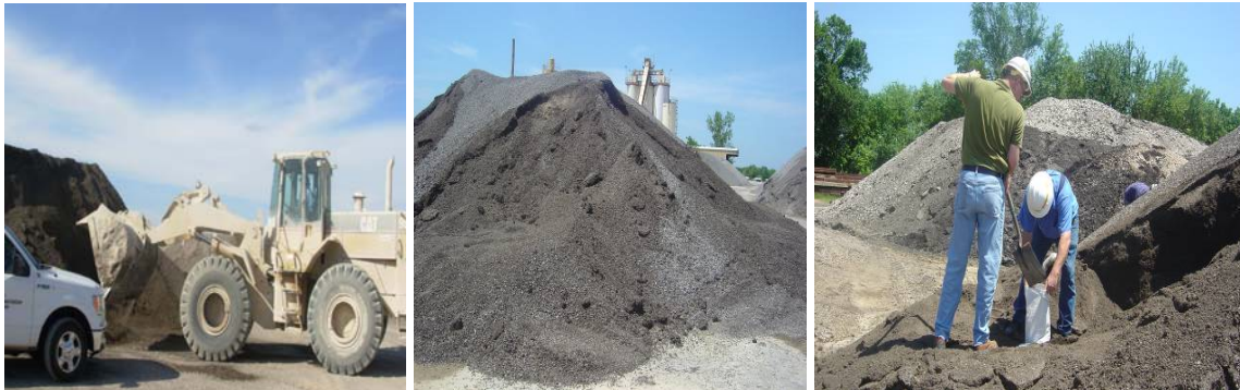
Figure 2-13. Sampling RAP Stockpiles.
