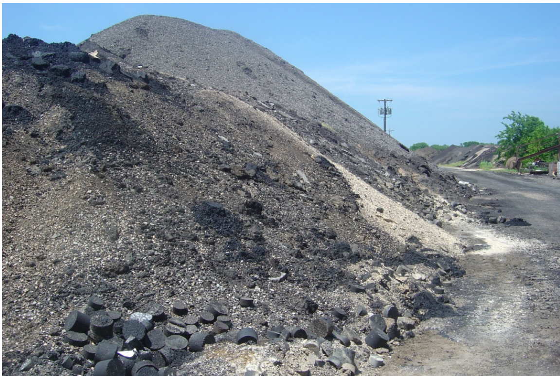
Figure 2-4. Blended RAP Stockpile.
