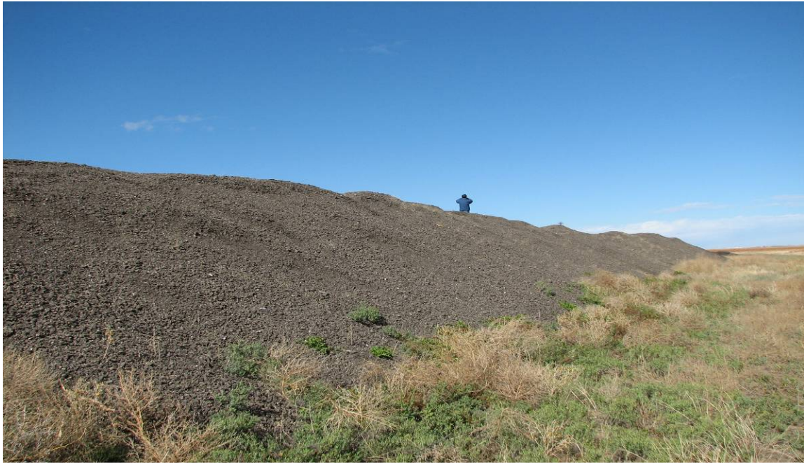
(a) Large, horizontal RAP Stockpile #1.
