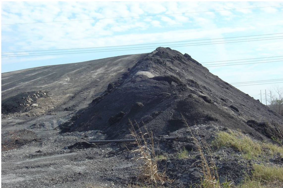
Figure 2-7. Trafficked and Compacted RAP Stockpile.
