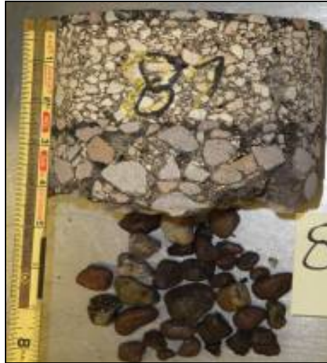
Figure 115. Core Taken from TRM 87 on IH 20.
