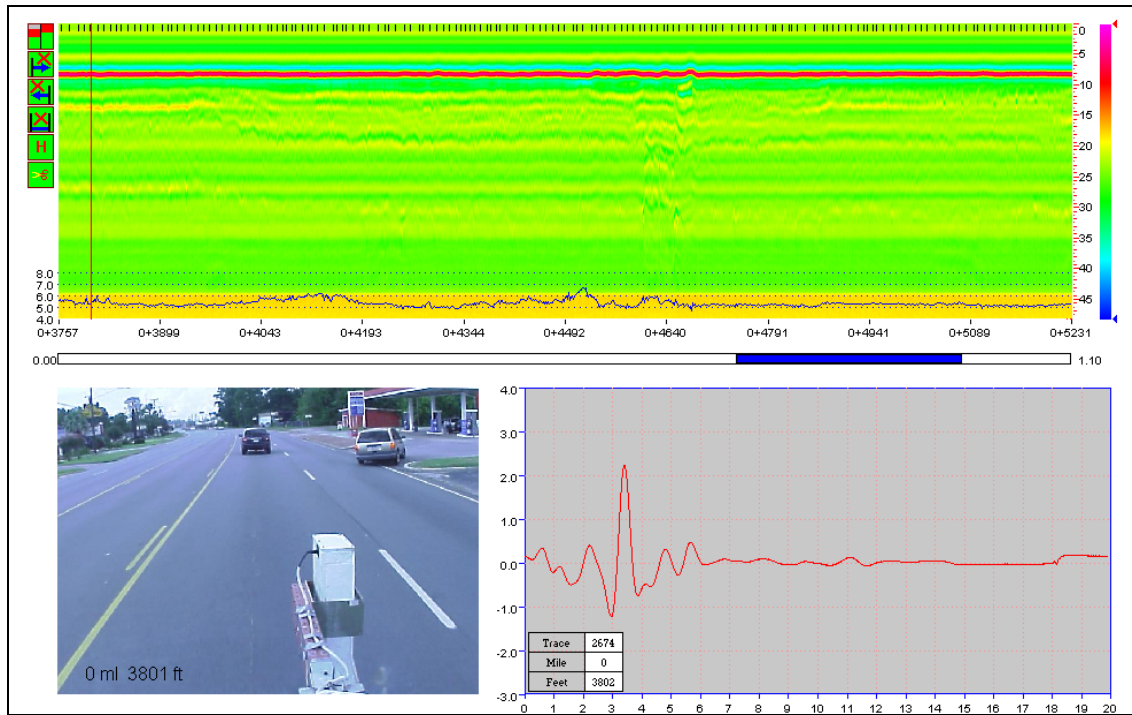
Figure 68. GPR Data on BU 59 after Five Years of Service.
