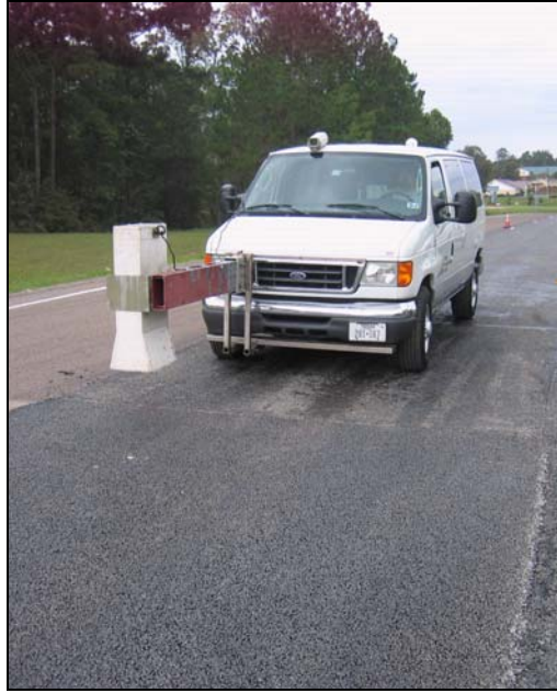
Figure 101. 1 GHz GPR Data Collection on US 190.
