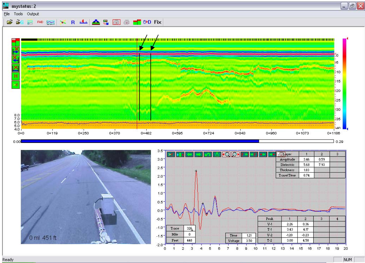
Figure 44. GPR Data on BU 290 after Seven Years of Service. Note: segregated areas identified during construction annotated with arrows.
