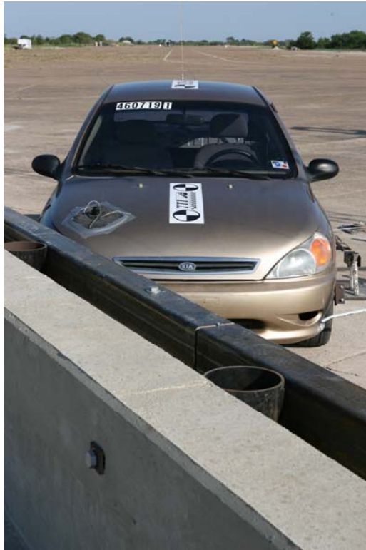
Figure 5.3. Vehicle/Installation Geometrics for Test No. 460719-1.
