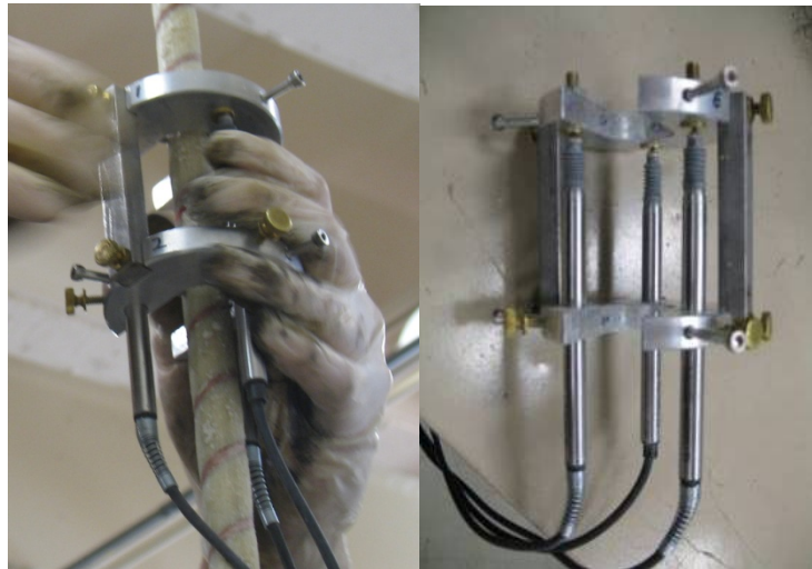
Figure 4-4. (a) LVDT Being Attached to GFRP Bar before Testing; (b) Close-up of LVDT Device.
