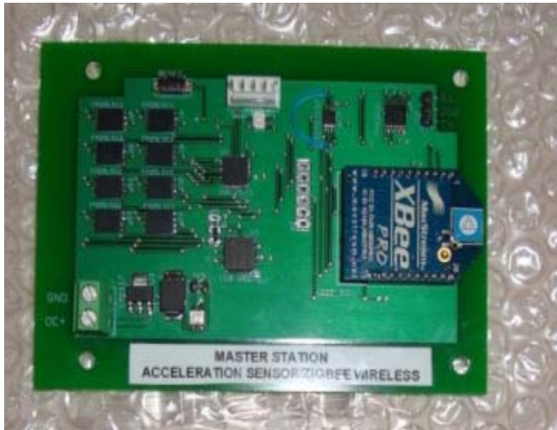
Figure 3-8. Circuit Board of Accelerometer.
