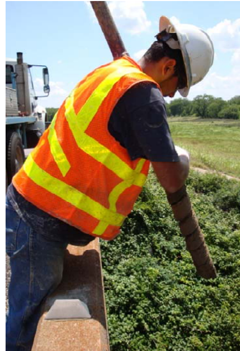
Figure 5-20. Remove Soil from the Drill Bit.
