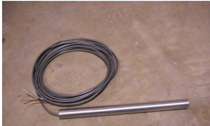
Figure C-11. Tethered Buried Switch Prior to Installation.
