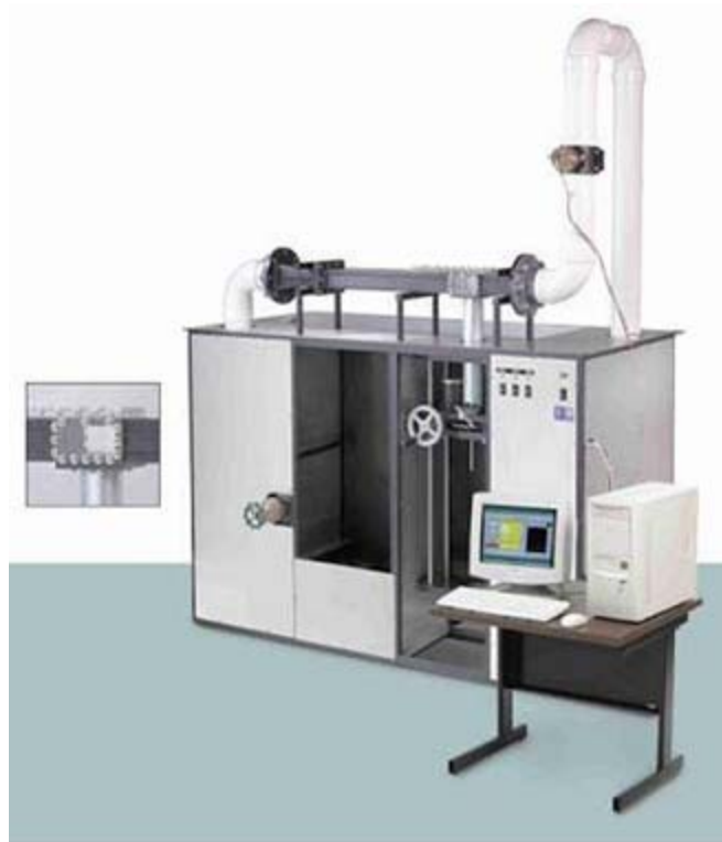
Figure 4-8. Erosion Function Apparatus.
