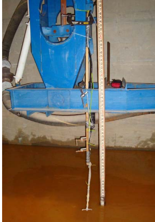
Figure 3-10. Acoustic Doppler Velocimeter Used in Laboratory.
