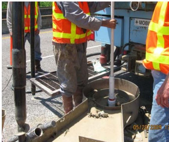
Figure 5-17. Lower the Float-Out Device.
