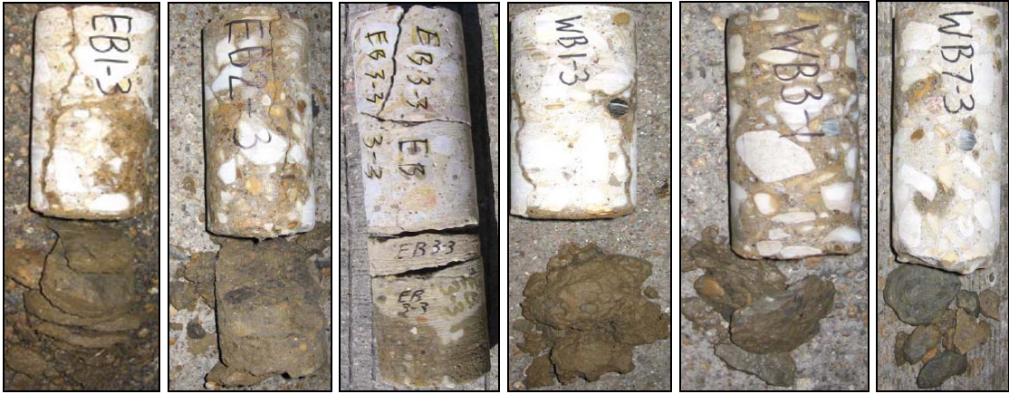
Figure 31. Cores of Sampled Section on IH 635.
