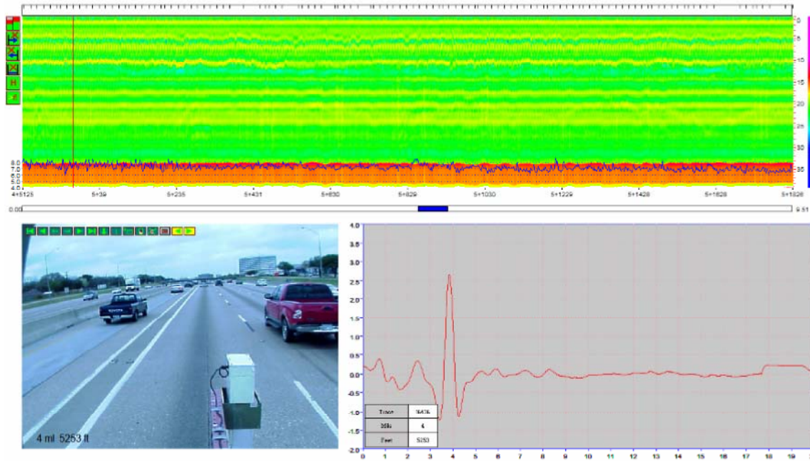
Figure 28. GPR Image of Sampled Section on IH 635.
