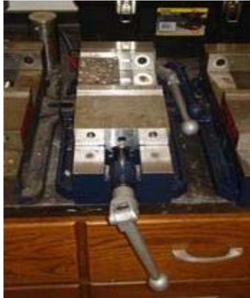
Figure 93. Magnetic Gluing Vice for Field Samples.
