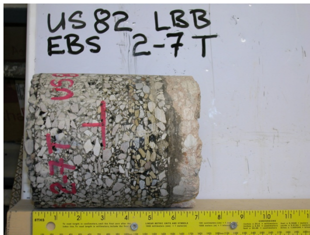
Figure 73. Sample Core with Seal Coat Treatment from US 82 Shoulder Section Collected in 2009.
