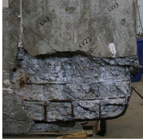
(b) Exterior Corner after Removal of Spalled Concrete (Opposite Face Shown in c)
