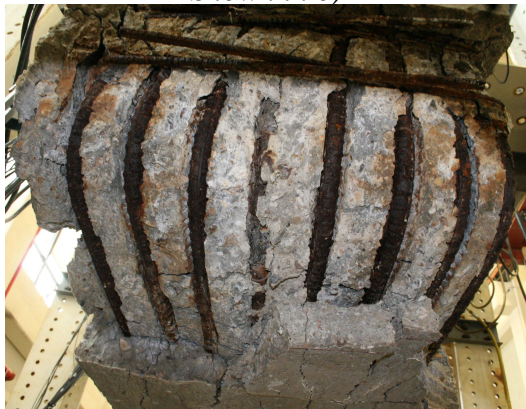
(e) Under Side of Exterior Corner Joint after Removal of Spalled Concrete
