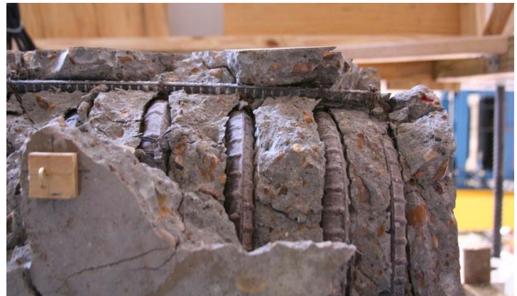
(f) Exterior face of the beam-column joint showing bulging of the U-bars and laterally displaced longitudinal steel
