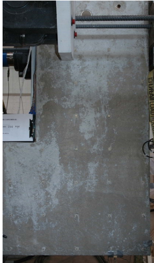
(b) Singly reinforced beam
