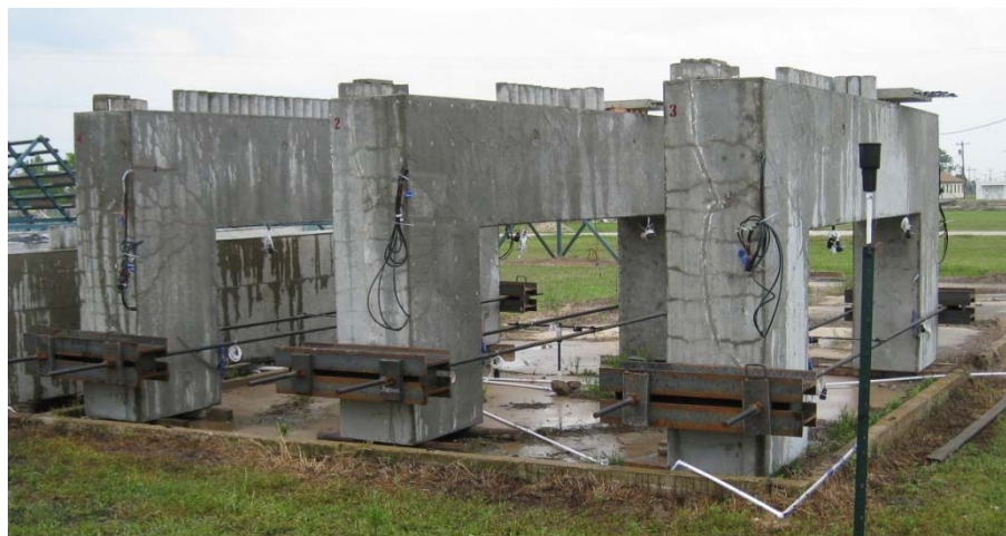
(c) C-Specimens exposed to environmental conditions
