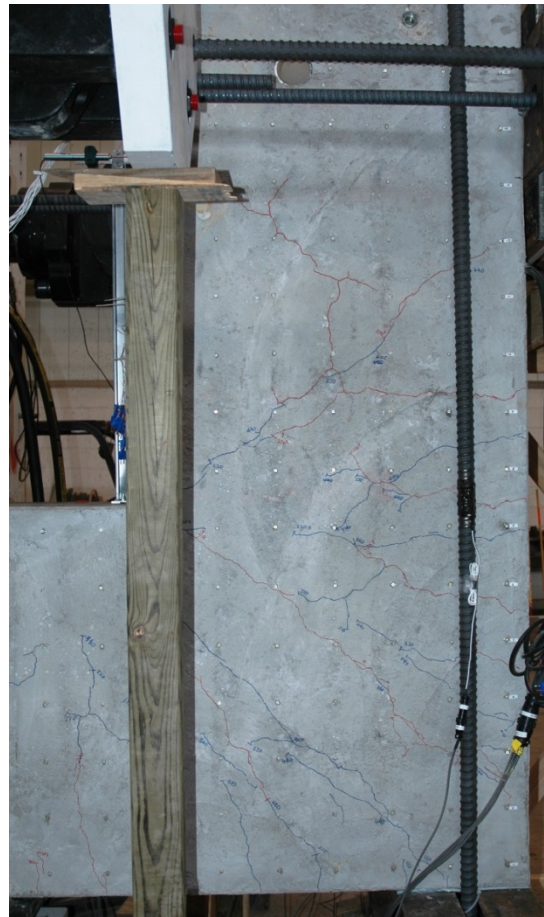
(b) Singly reinforced beam
