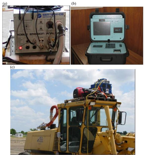
Figure 16. Emission Measurement Instruments: (a) SEMTECH-DS Unit, (b) Axion Unit, and (c) Both Units along with EFM Installed on a TxDOT Grader.
