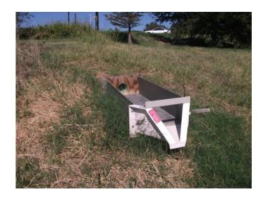
Figure 10. H-Flume Installed at the Effluent Location to Measure Flow.
