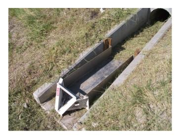
Figure 9. H-Flume at the Influent Location to Measure Flow.
