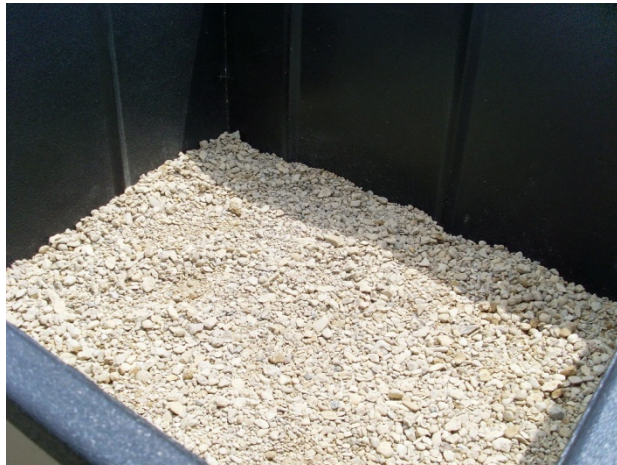
c. gravel layer (8 inches in depth)
