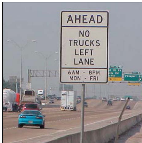
Figure 28. Truck Lane Restriction Sign on Texas Freeway.
