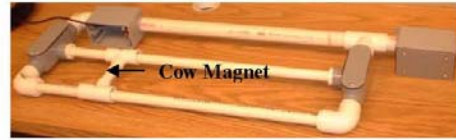
Figure 5. Ambient Magnetic Field Adjustment Device 2 for Single 701 Traffic Sensor.
