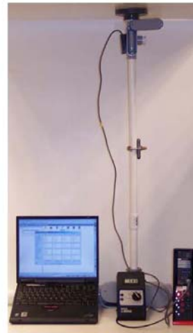
Figure 4. Using 701 Traffic Sensor Attached to C924 Vehicle Detector Combined With C900 CS to Measure Response to Vehicles
