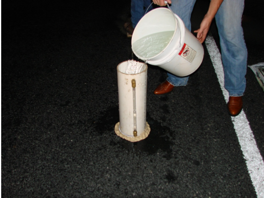
Figure 14. WFV On-Site Test Setup.
