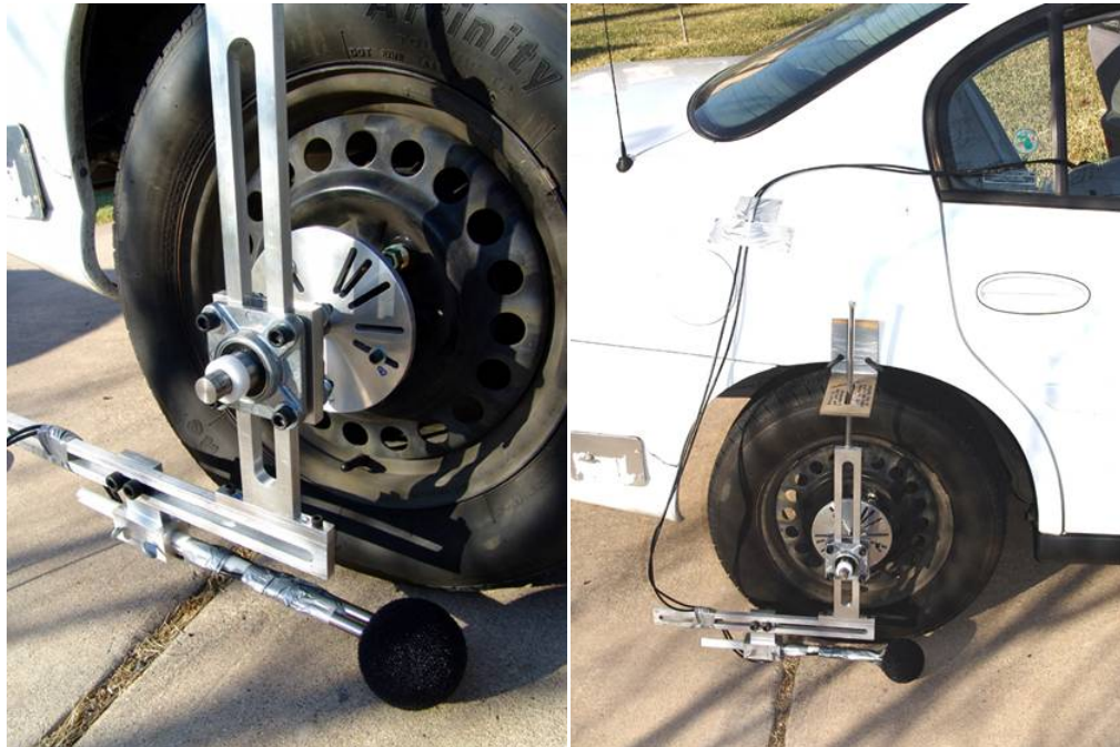
Figure 6. Single Probe Fixture with Microphone Pair in Horizontal Position.
