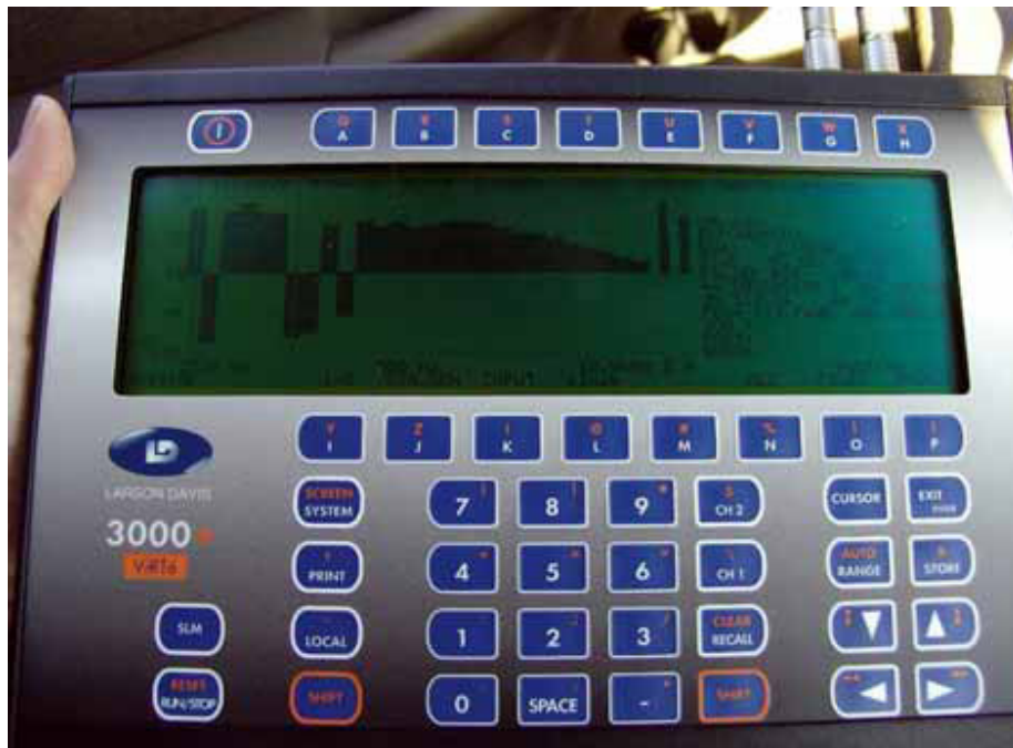
Figure 9. Larson Davis 3000+ Sound Intensity Analyzer.
