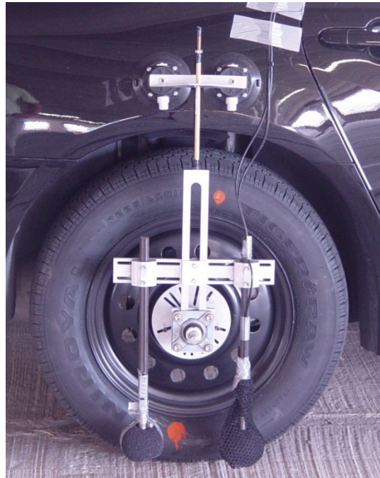
Figure 7. New OBSI Fixture.
