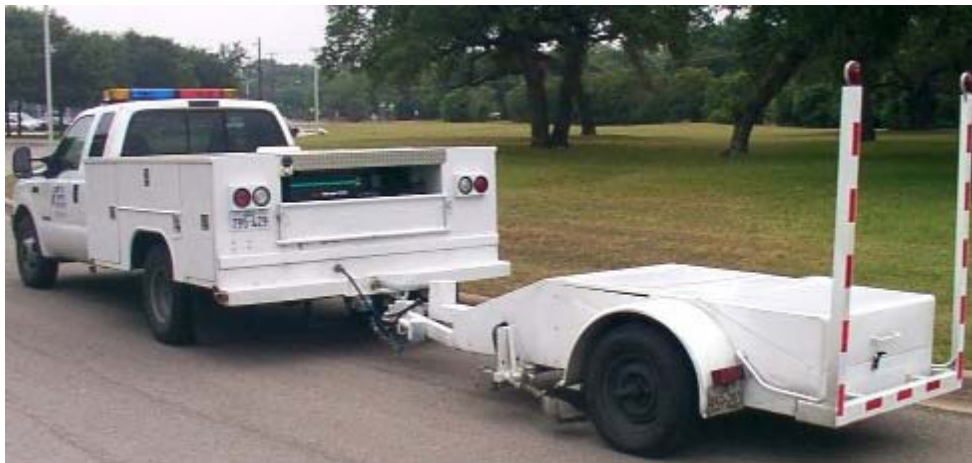
Figure 19. Two-Wheeled Trailer with Left Wheel Path Locking Tire.
