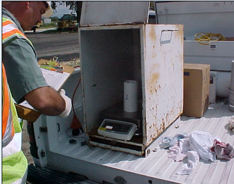
Figure 6 – Weighing Cylinders to Nearest Gram
