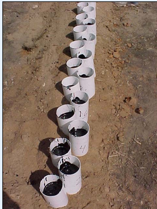
Figure 5 – Cylinders \frac{3}{4} Filled with Asphalt
