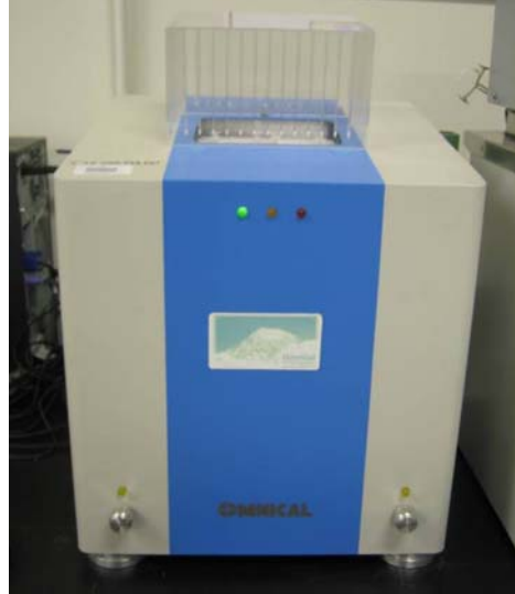
Figure 3.9. Conduction Calorimeter for Heat of Hydration.
