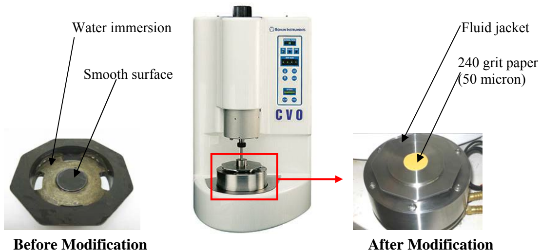
Figure 3.3. Modified DSR with the Fluid Jacket System.
