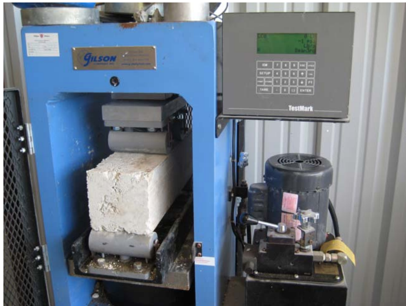
Figure 5-4. Modulus of Rupture Test Set-Up.
