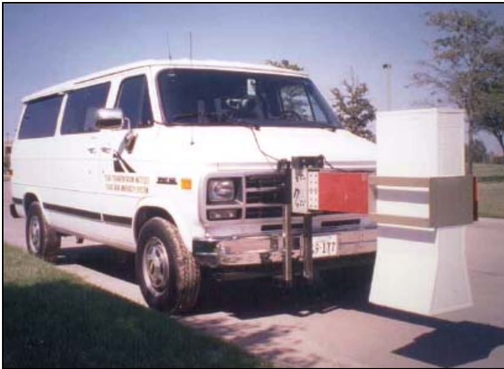
Figure 6-4. Air-Coupled GPR System Mounted on TTI Van.
