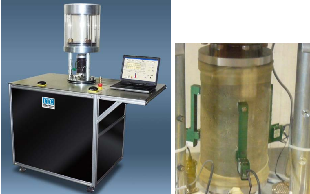
Figure 7-3. New Generation of HMA Test Equipment with Automated Sensors.
