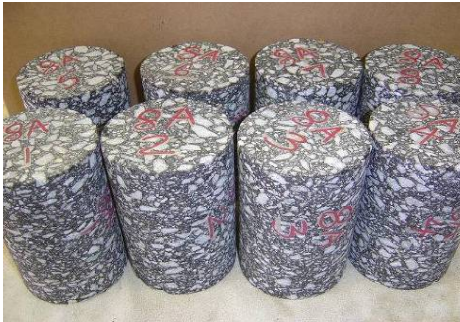
Figure 3-8. Examples of Prepared Specimens for Dynamic Modulus Test and Repeated Load Test.
