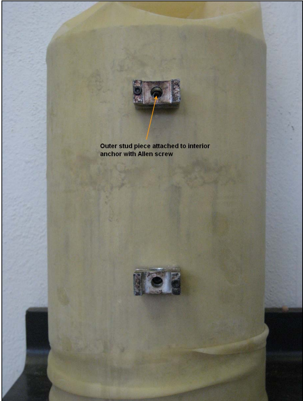
Figure B4. Outer Stud Piece Attached to Inner Piece with Allen Screw.
