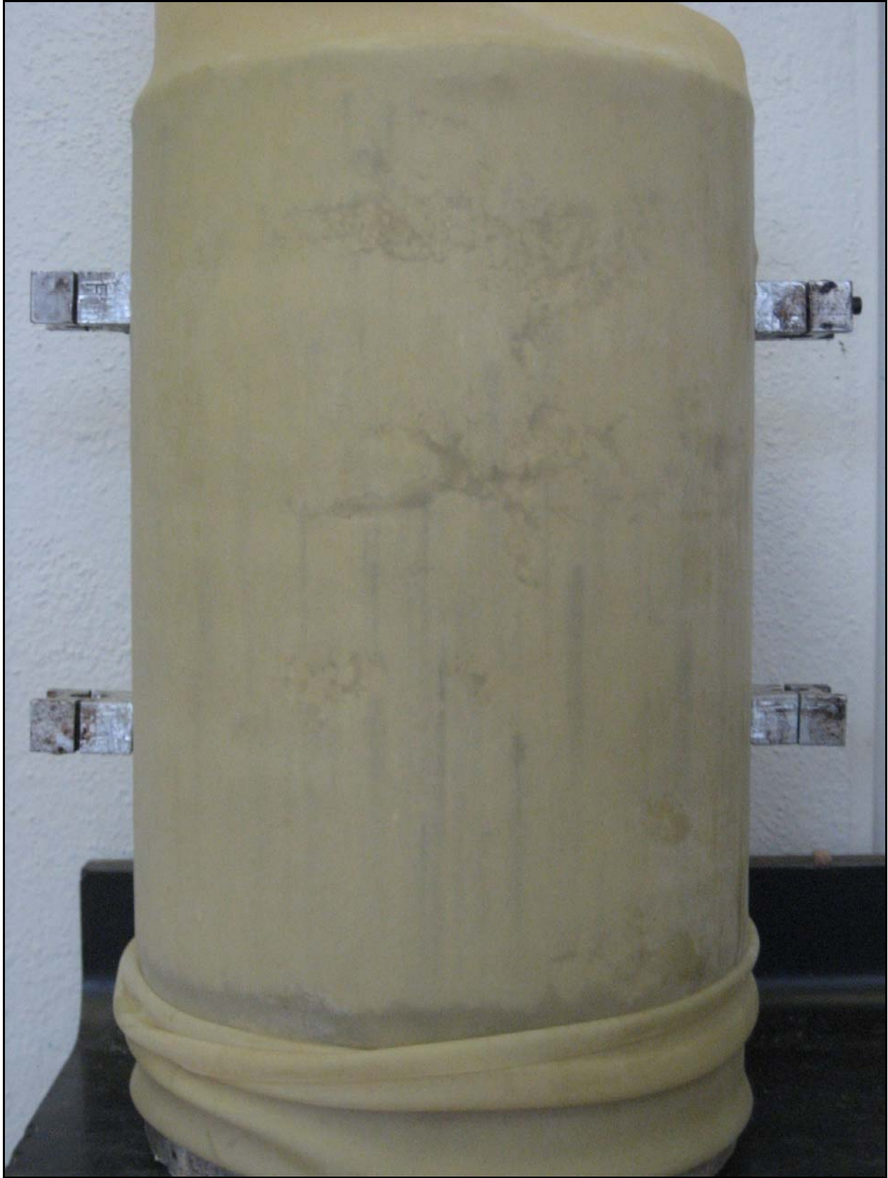
Figure B5. Molded Specimen with Stud-Mounted LVDT Holders.
