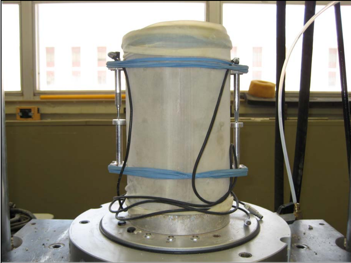
Figure B6. Test Setup using Rubber Bands to Hold LVDTs.
