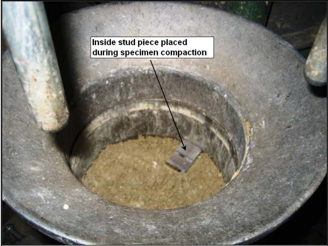
Figure B3. Inner Stud Piece Placed inside the Specimen during Compaction.
