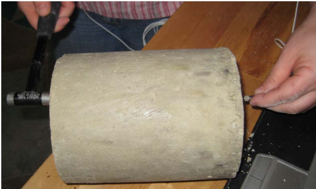
Figure 5-3. Seismic Modulus Test Being Conducted.
