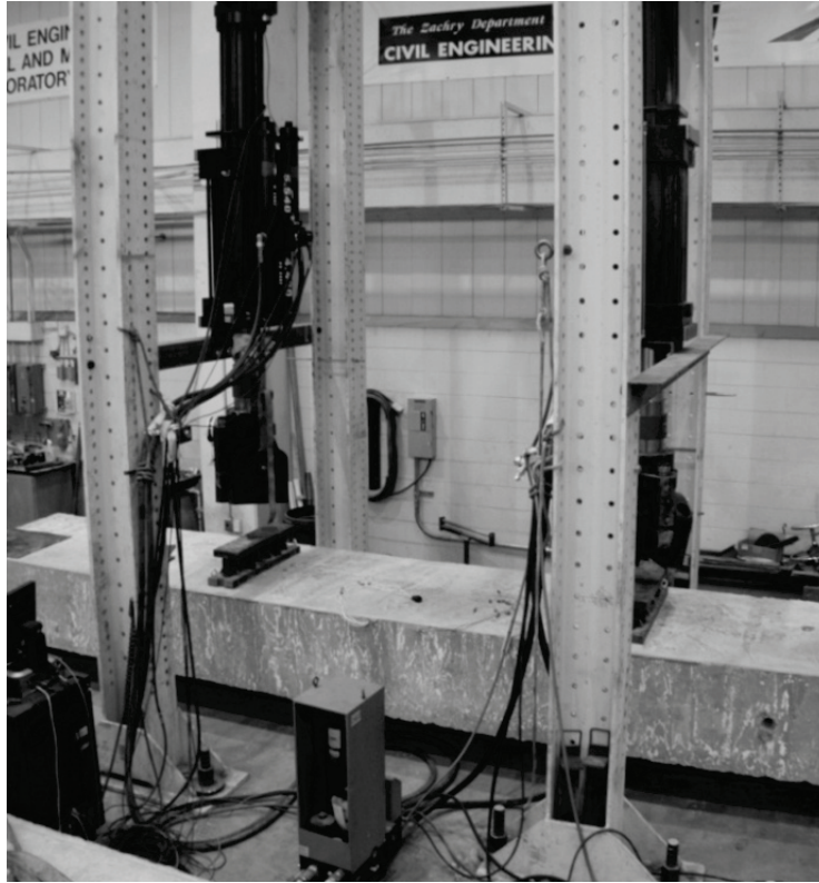
Figure 4-7. Specimen in the Four-Point Test Setup.
