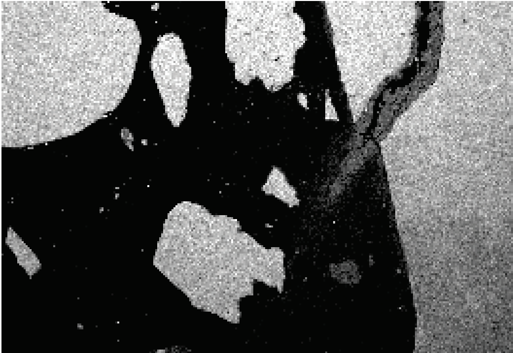
Silica dot map illustrating siliceous aggregates and silica rich gel
