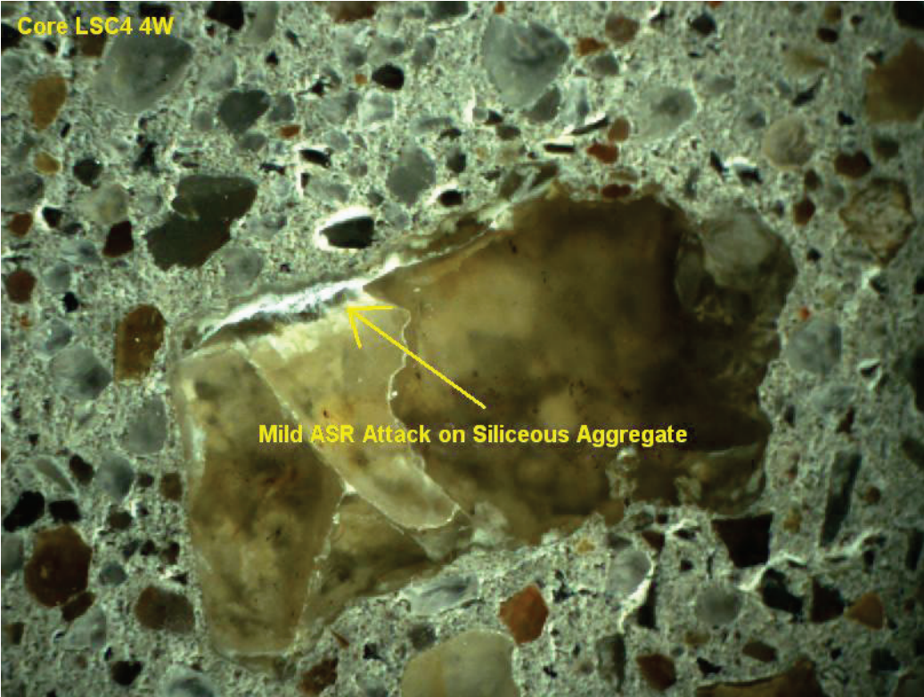
Mild ASR distressed aggregate
