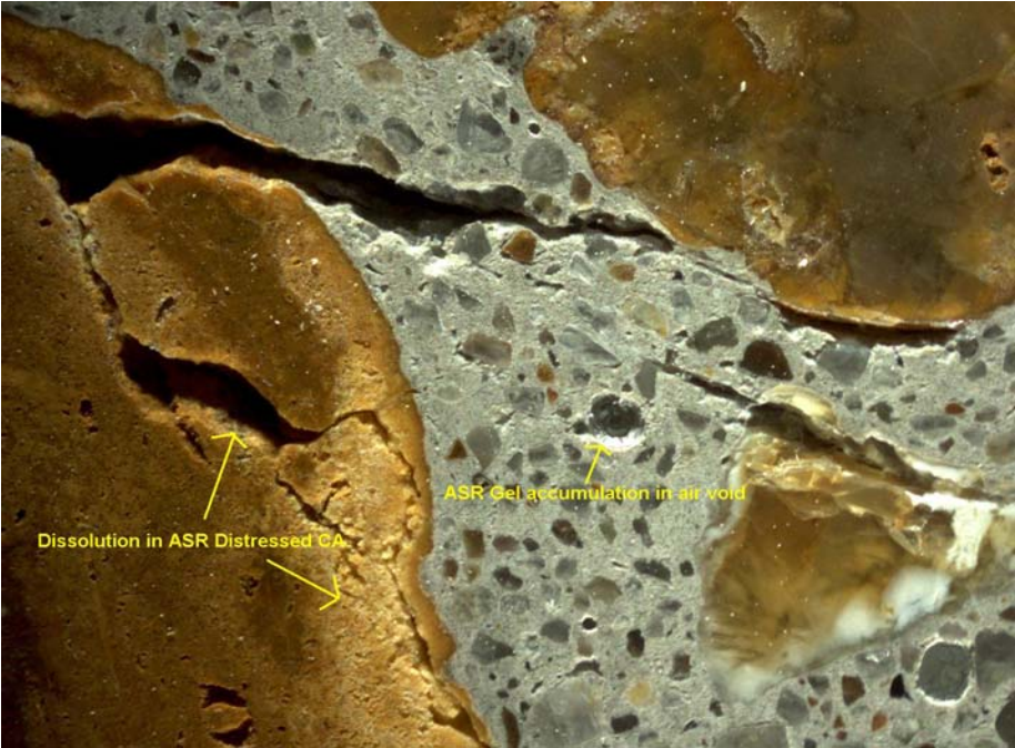
Image illustrating ASR distress features in core 5-2
