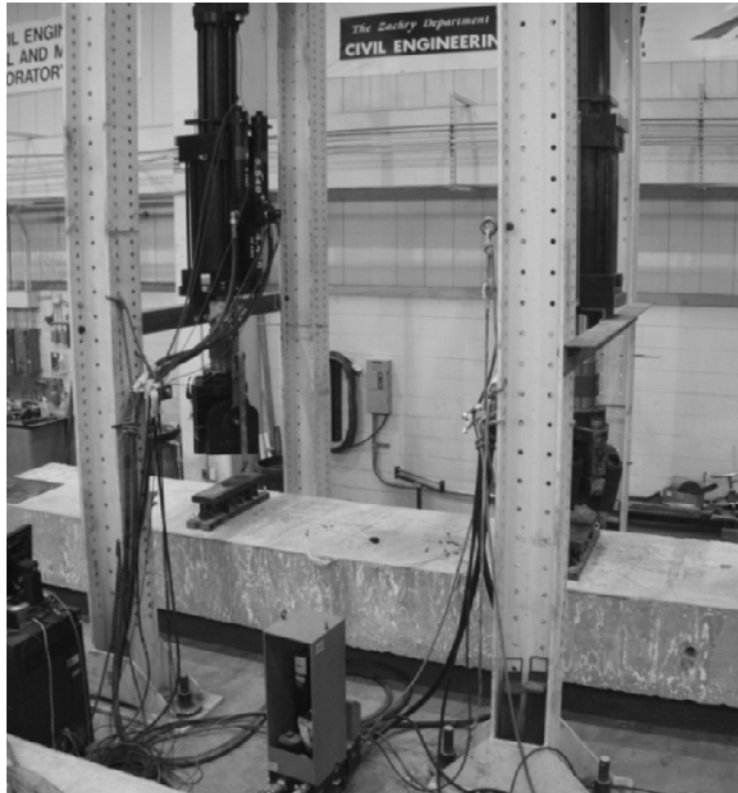
Figure 5-4. Specimen in the Four-Point Test Setup.
