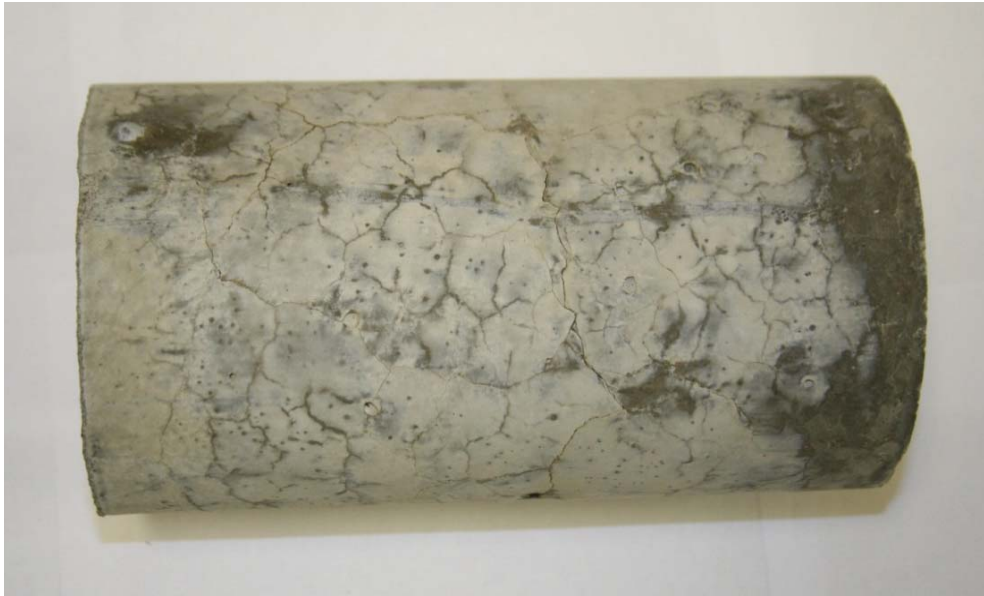
Figure 5-15. Cracking of a Cylinder Stored at the Riverside Campus.
