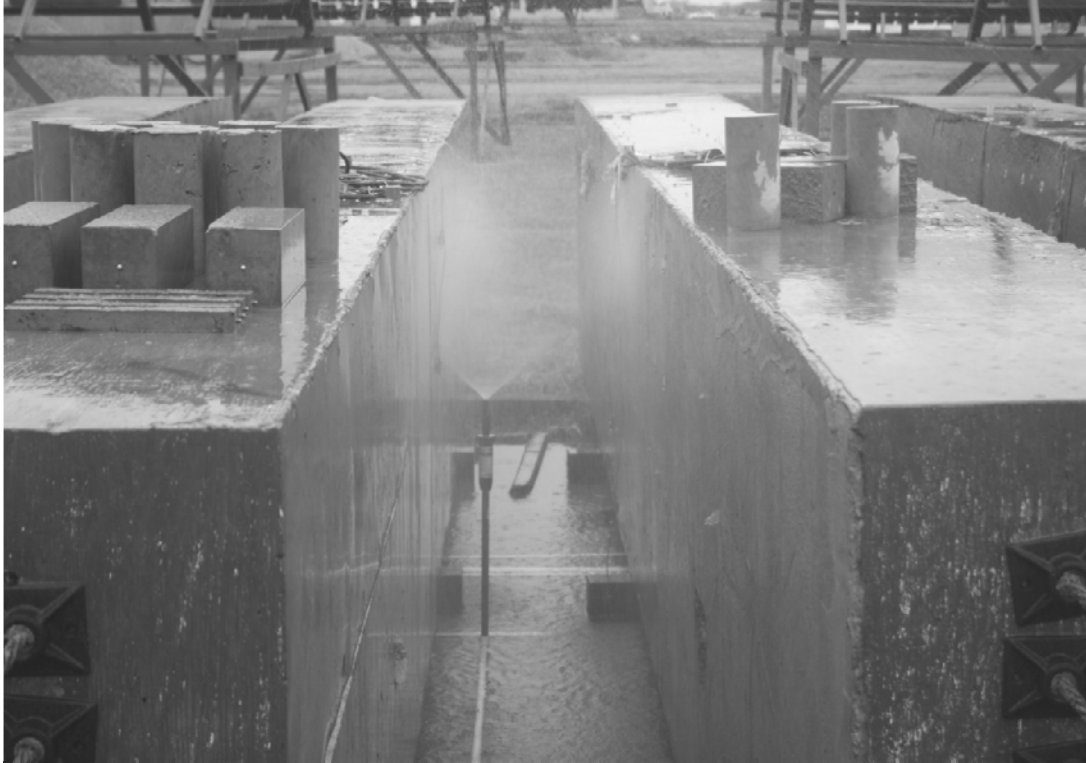
Figure 3-4. Sprinkler System between Two LSC Specimens.
