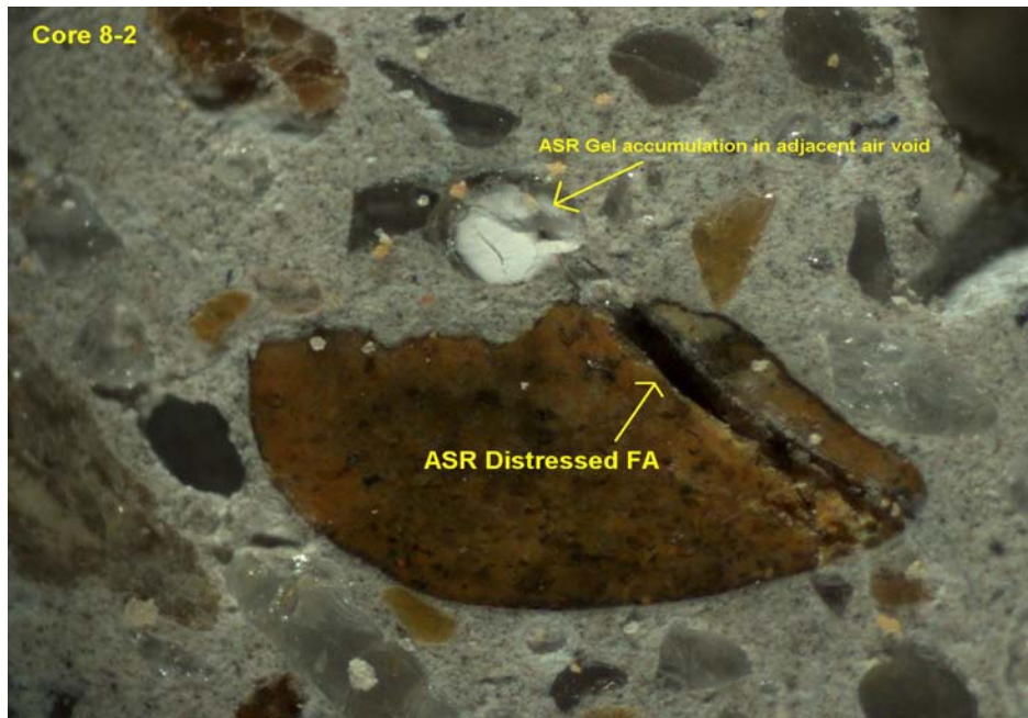
Image illustrating ASR distress aggregate
