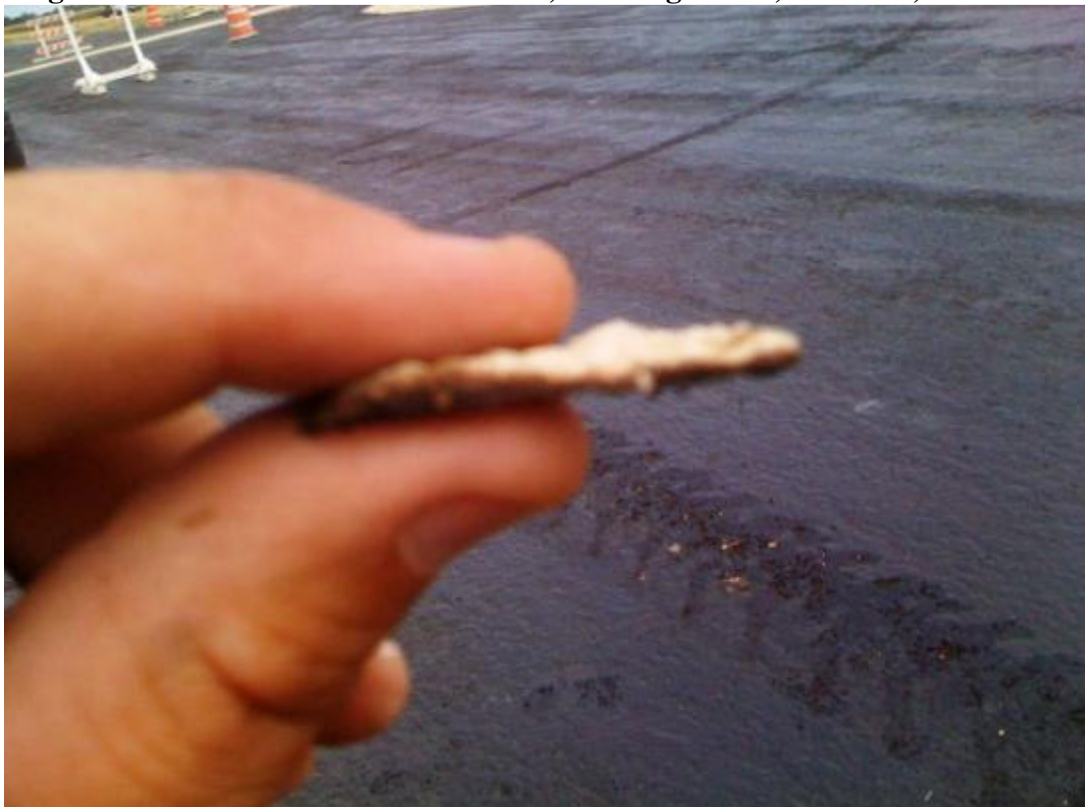
Figure C-5. Penetration of 1/16 of an Inch.
