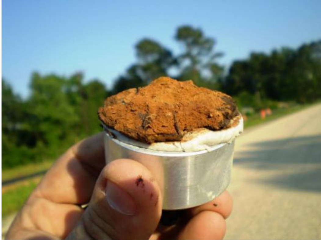
Figure 20. Atlanta, FM 134, MC-30. Pull-off. Fines Only.
