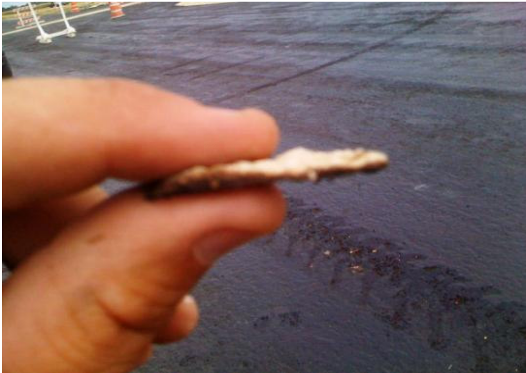
Figure 9. Penetration of 1/16 of an Inch.
