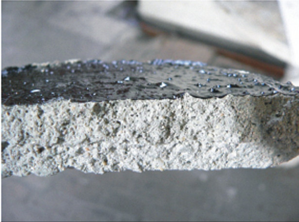
Figure C-1. No Penetration with Normal Emulsified Asphalt (a suspension of asphalt in water) (After SABITA, 2006 ).
