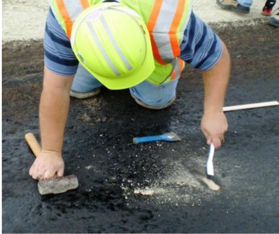
Figure 8. Penetration Measurement, Showing Chisel, Hammer, and Scale.
