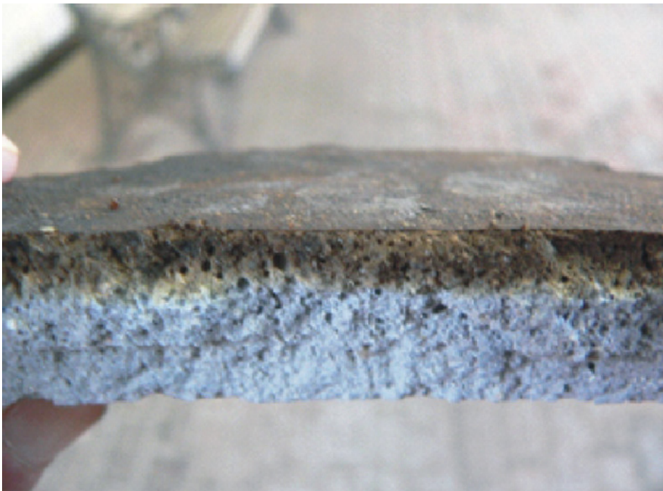
Figure C-2. Penetrating Effect of Inverted Asphalt Emulsion Prime (a suspension of water in asphalt) (After SABITA, 2006 ).
