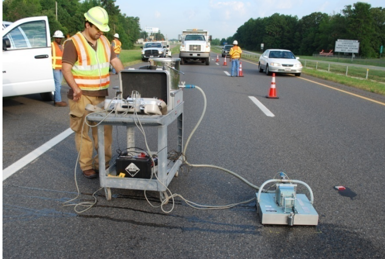
Figure 5. Layout of the Measurement Section: DFT Measurement.
