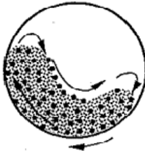
Figure 32. Mechanism of Aggregate and Steel Balls Interaction in Micro-Deval Apparatus.
