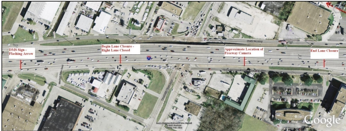
Figure A-16. Work Zone Layout for Site 13.
