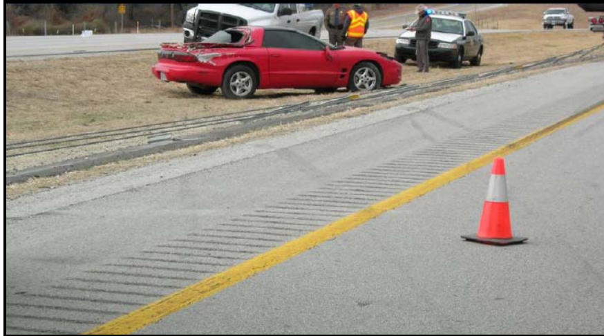
Figure 4-11. Example of a Passenger Car Cable Barrier Penetration Event.
