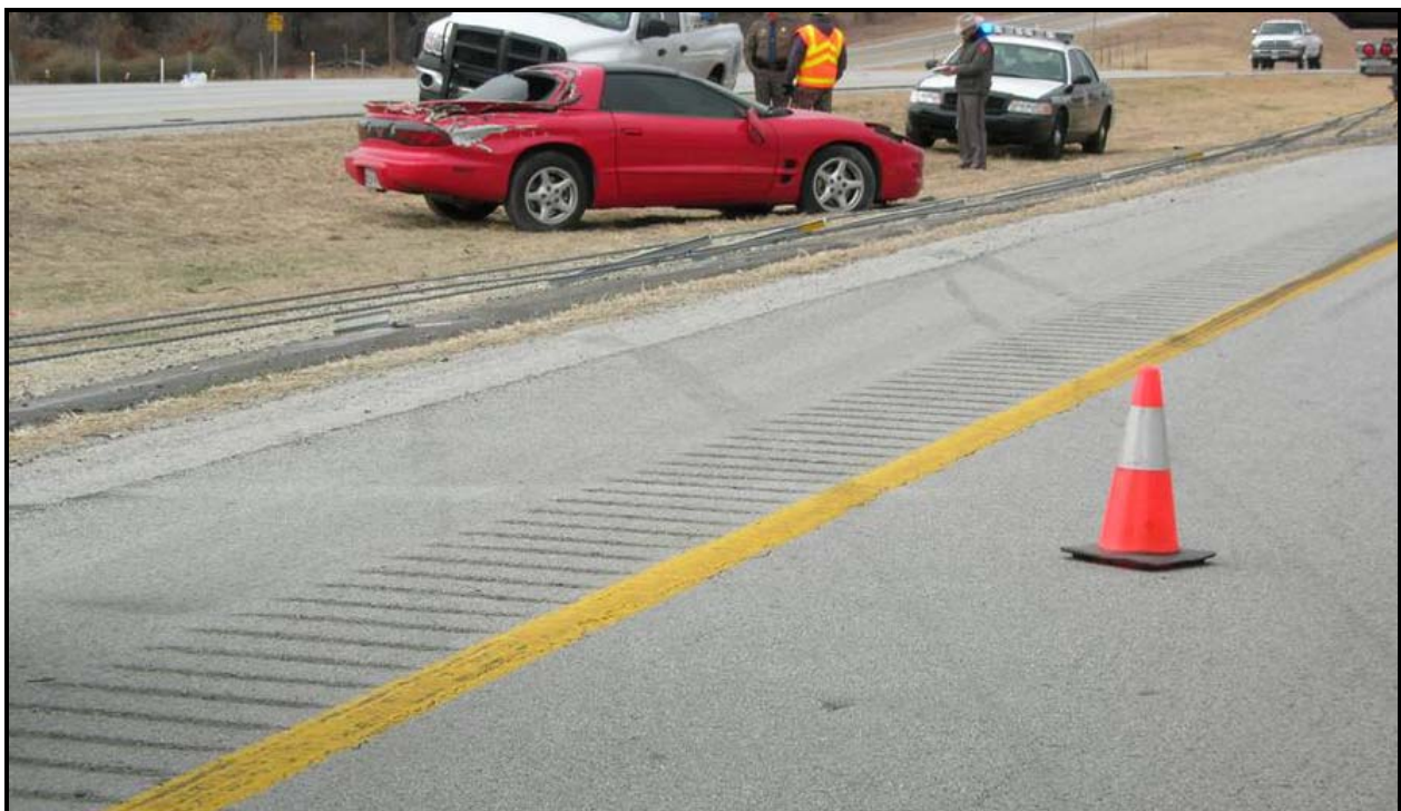
Figure 5-7. Non-Standard Impact Conditions: Low Bumper and High Impact Angle.
