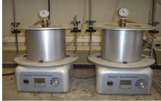
Figure 2. Specific Gravity Testing Using Metal Vacuum Pycnometer.
