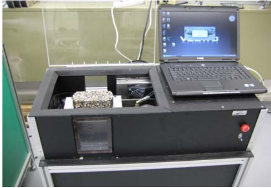
(a) Overlay Testing
