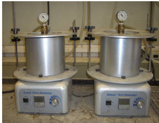
Figure 50. RICE Testing using Metal Vacuum Pycnometer.
