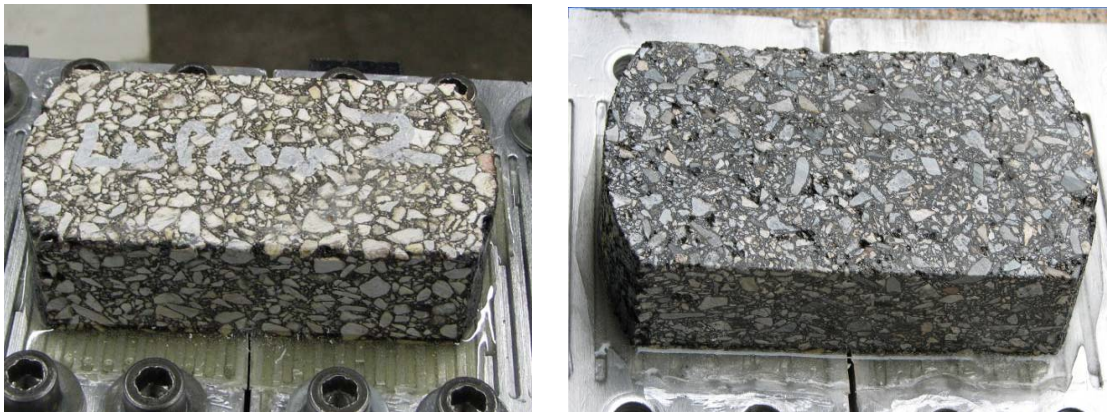
Figure 8. Lufkin's Traditional Maintenance Type D Mix (Left) CAM Mix (Right).
