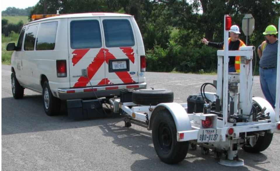
Figure 5.32. TxDOT's Falling Weight Deflectometer (FWD) Testing Equipment.
