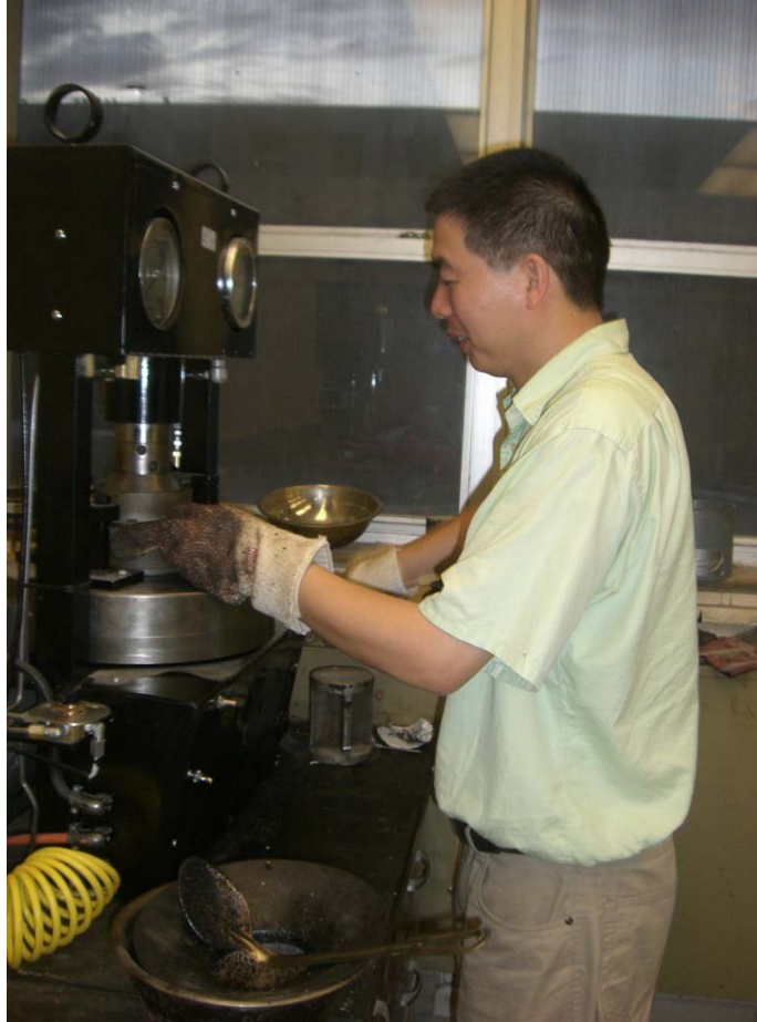
Figure 2.5. Compacting WMA Mixtures in the Texas Gyrotory Compactor (TGC) at TTI.
