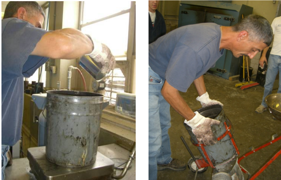
Figure 2.4. TTI Technicians Performing WMA Mixture Designs at TTI Laboratory.
