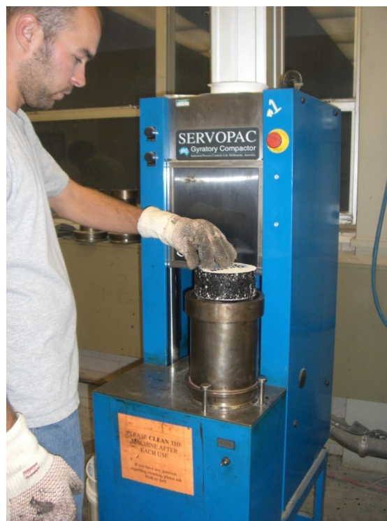
Figure 2.12 Compacting Hamburg Wheel Tracking Test (HWTT) Specimens in SGC.
