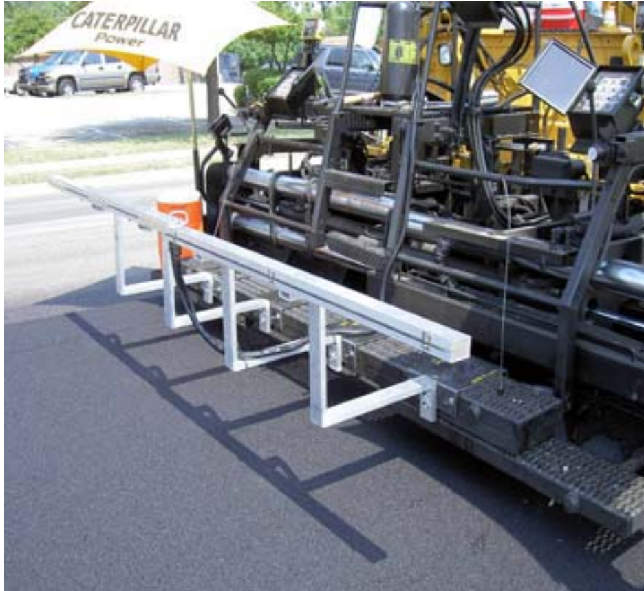
Figure 5.20. Pave-IR Installed on Paving Machine.
