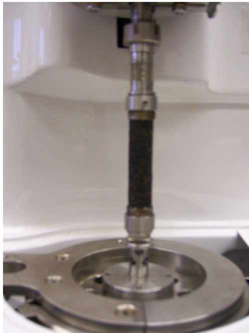
Figure 4.4. Asphalt Mastic Specimen in DMA Testing Apparatus.
