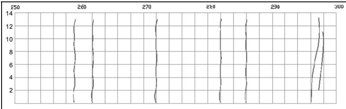
Figure C46. Visual Survey Chart for I-35 R1 Lane (250 to 300 ft, 07/15/2008 survey).
