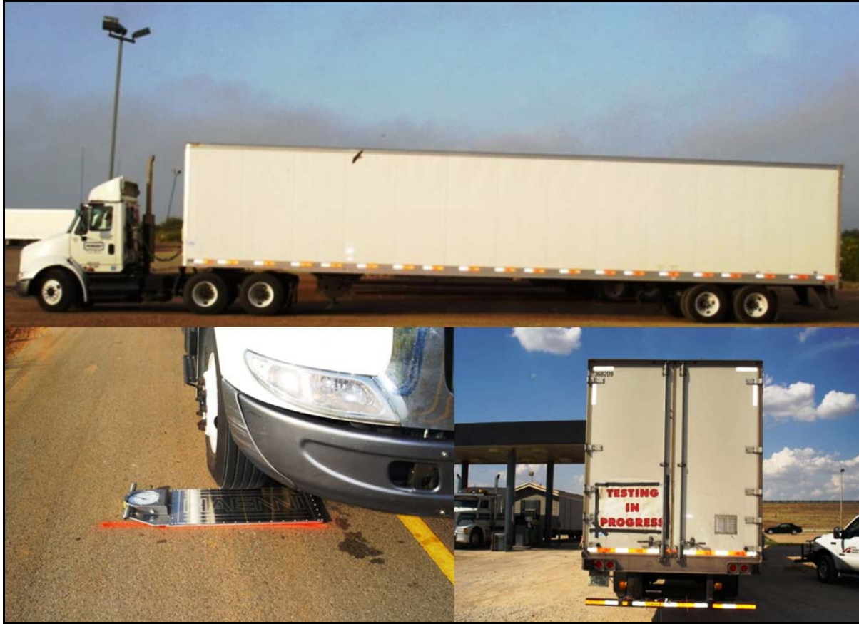
Figure 3.1. Test Vehicle Used for Verifying LTPP WIM Smoothness Criteria.
