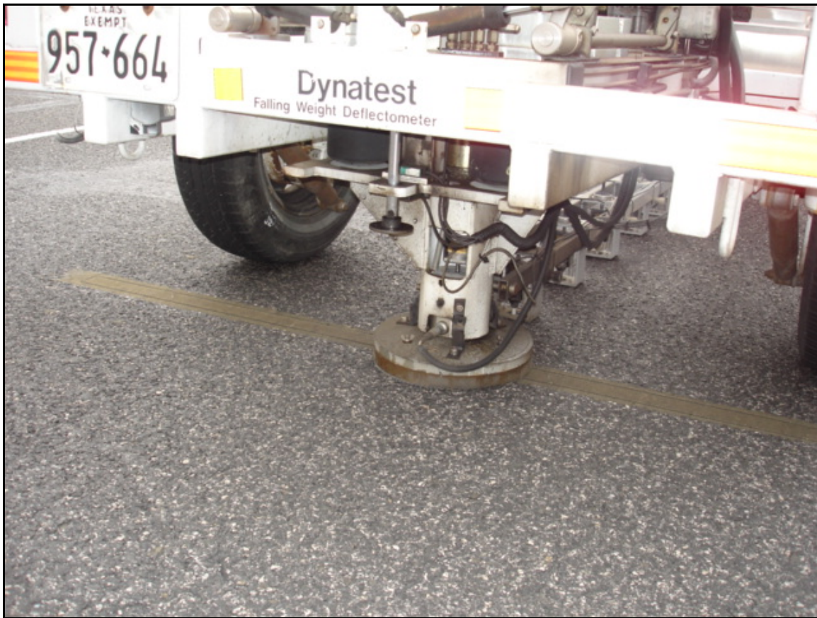
Figure 3.2. FWD WIM Sensor Testing.
