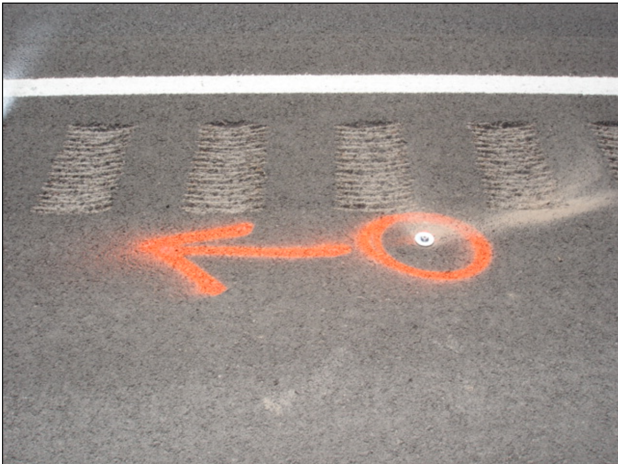
Figure E4. Marker Placed at End of Proposed WIM Sections on Westbound Lanes.
