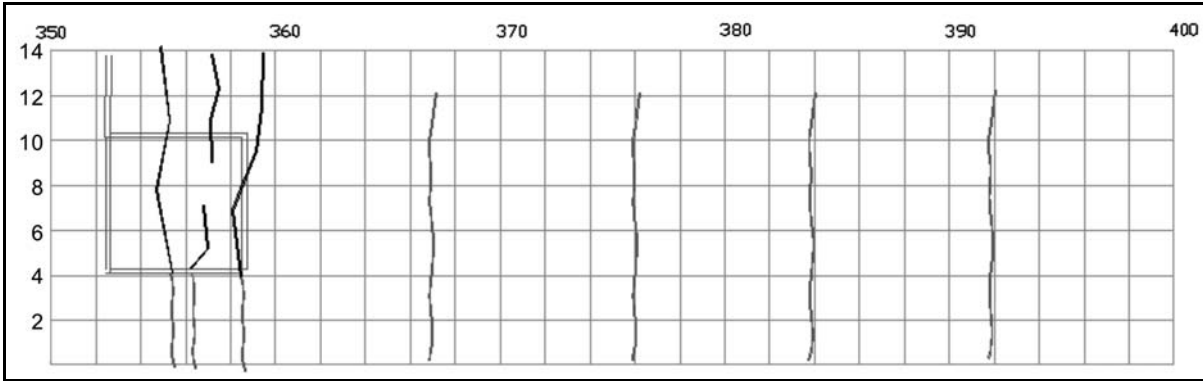
Figure C18. Visual Survey Chart for I-35 R2 Lane (350 to 400 ft, 07/20/2007 survey).
