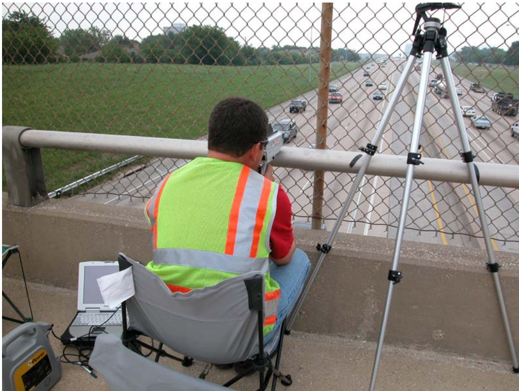
Figure 3-16. Spot Speed Data Collection at Site 1.
